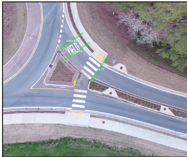
Figure 12. Photo. Typical position of approach monitoring gates used to capture vehicle attributes as drivers modify driving to enter the roundabout.
