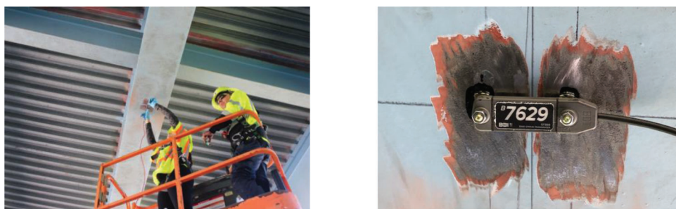
Figure 3.2 Researchers adhering a strain gauge to the bottom flange of Asset 020-20-07229 (left) and an adhered gauge (right).
