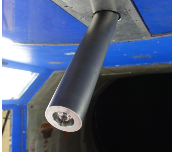
Figure 3. Photo. View of the upper dummy section with the two-component force sensor installed.
