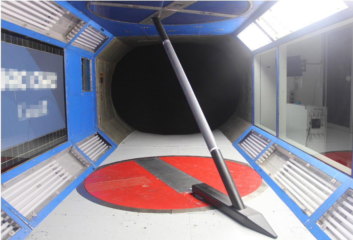
Figure 4. Photo. View from downstream of the cable model inclined at 45 degrees.
