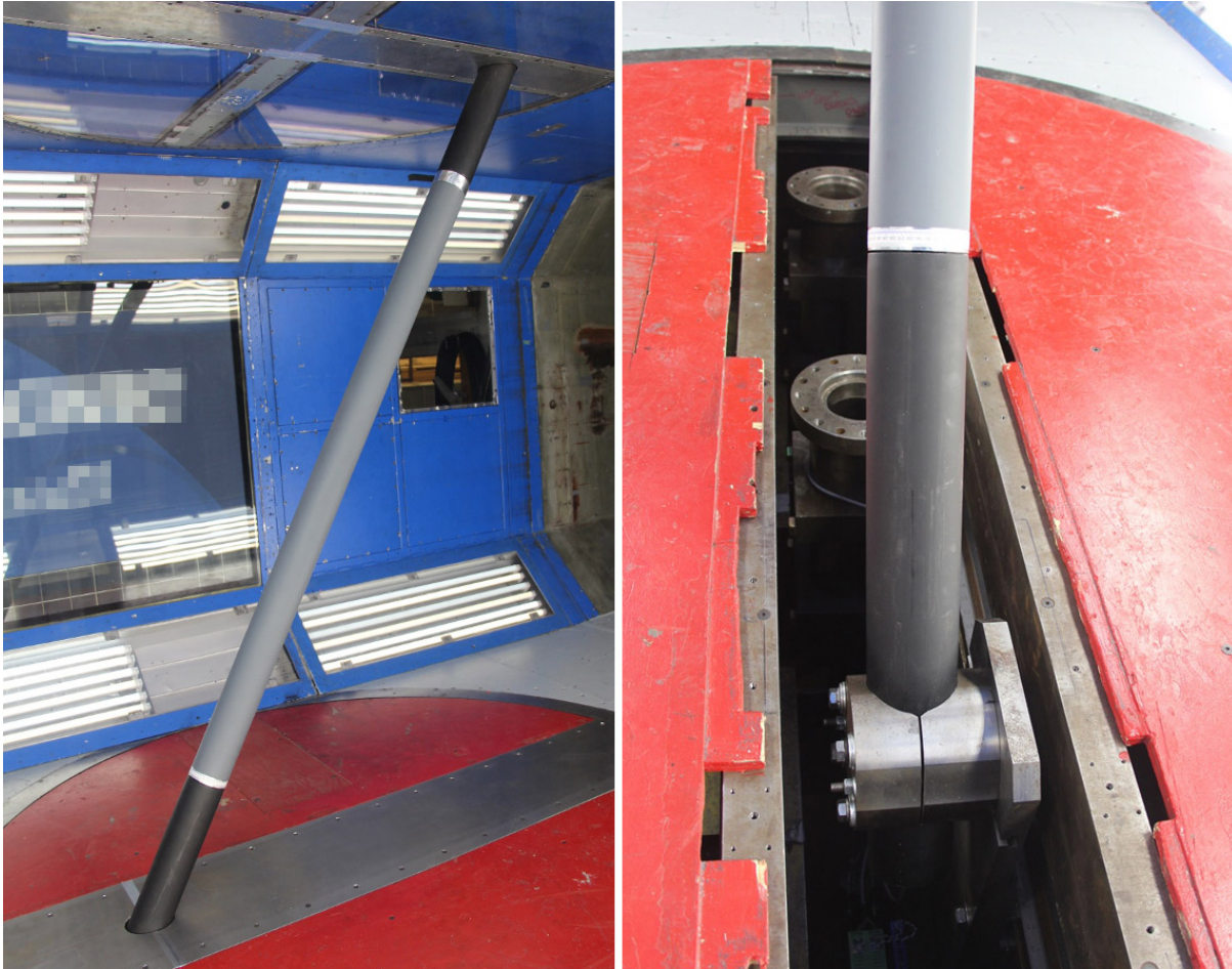
Figure 2. Photos. Views of the cable model and the lower dummy section interface with the floor turntable of the 2- by 3-m wind tunnel.
