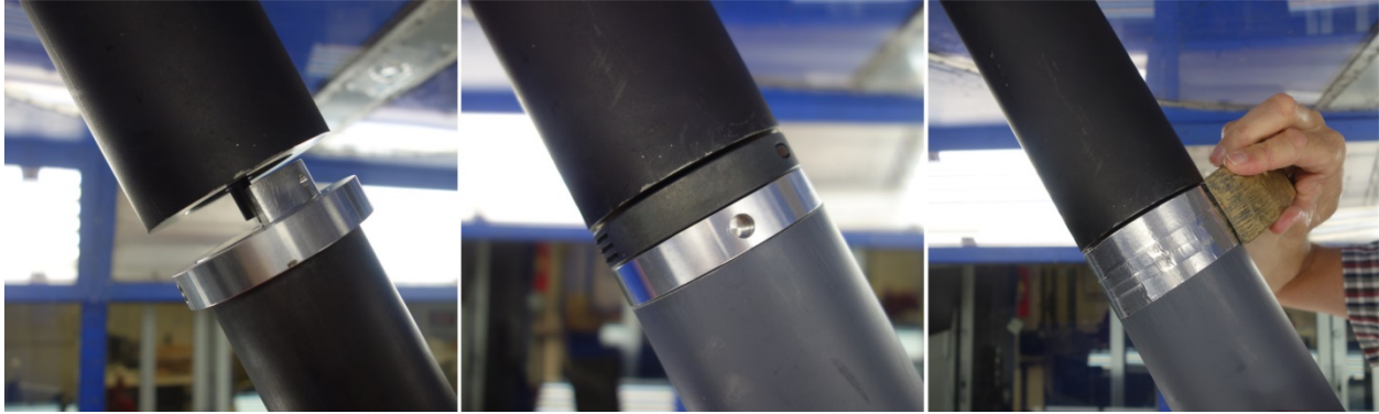
Figure 5. Photos. Views of the interface between the central part of the model and the upper dummy section.
