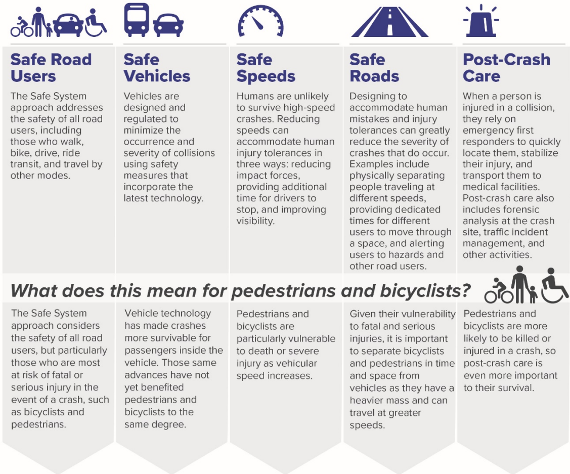
Figure 1. Graphic. The five elements of the Safe System approach and their relevance to pedestrians and bicyclists (FHWA, 2020a).
