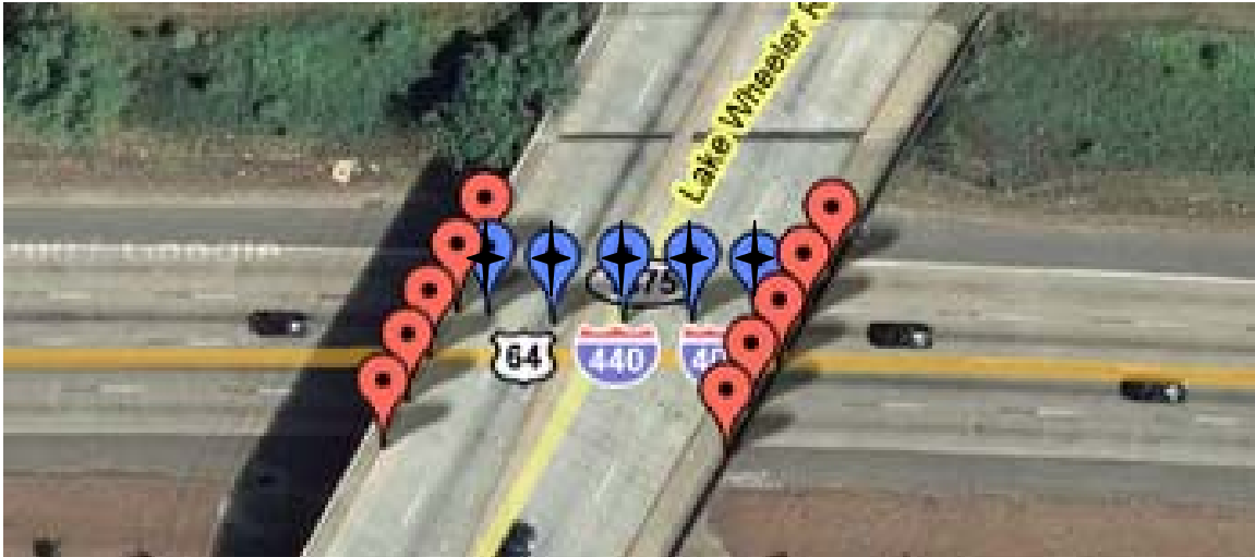
Figure 4.15. Survey and Geo-3D measurement locations for Lake Wheeler Road bridge.
