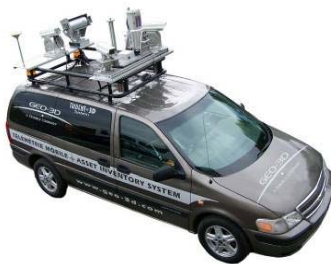
Figure 4.8. Geo-3D mobile data collection vehicle.
