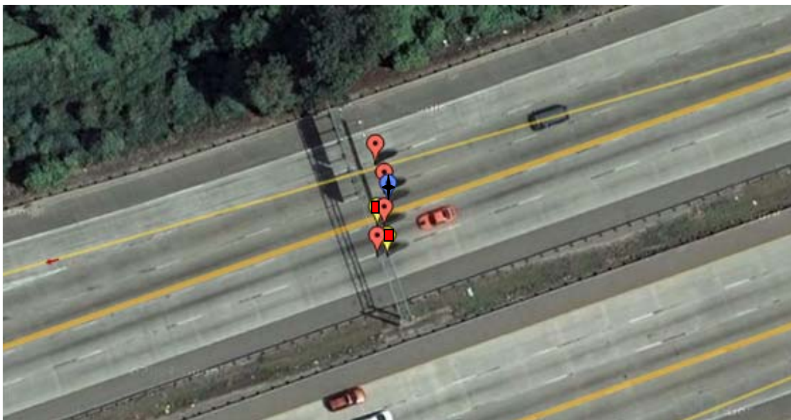
Figure 4.17. Measurement locations for South Saunders Street exit sign.
