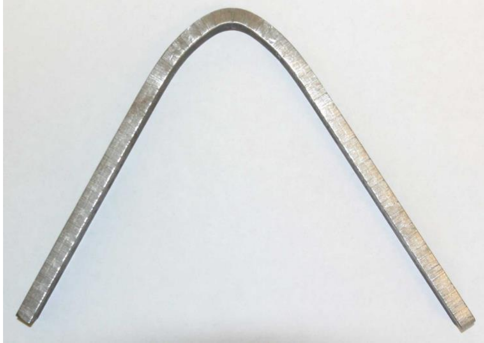
Figure 36. Post-test photograph of a specimen cut out from the collision post, across the shelf tab weld
