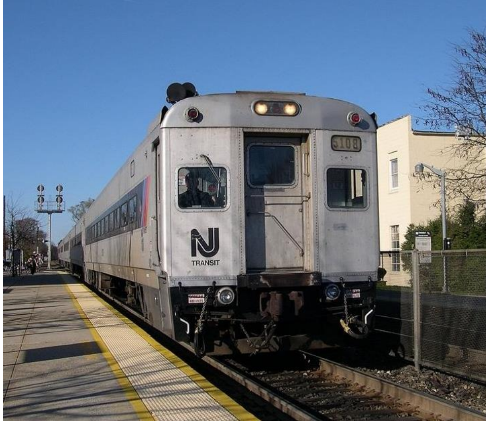
Figure 1. An example of a cab car in which the operator is positioned immediately adjacent to the vehicle end
