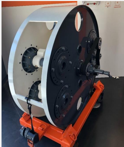
Figure 38: Cut-out model of Hamm asphalt roller drum
