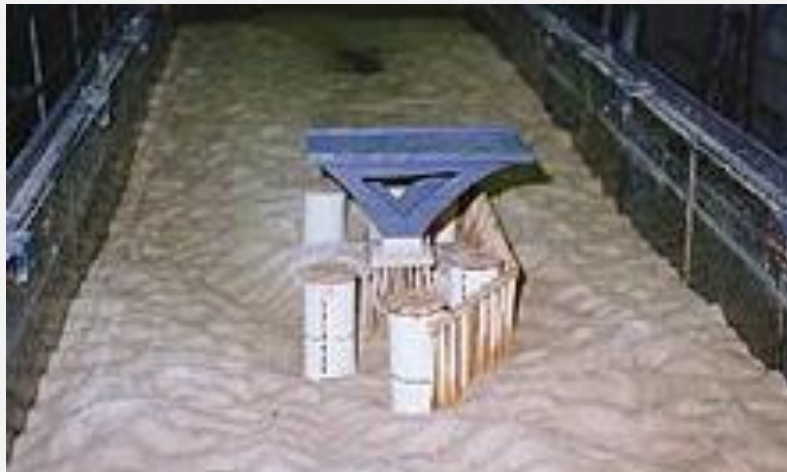
Figure 37: Scour testing on Woodrow Wilson Bridge model
