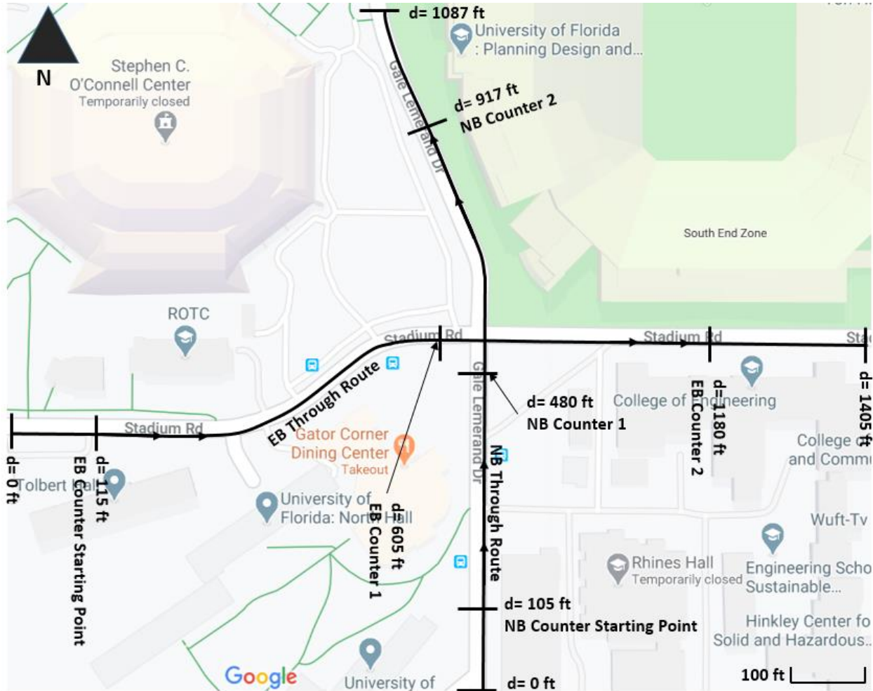
Figure 5-1 Schematic Representation of EB-Through and NB-Through and their Respective Counters
