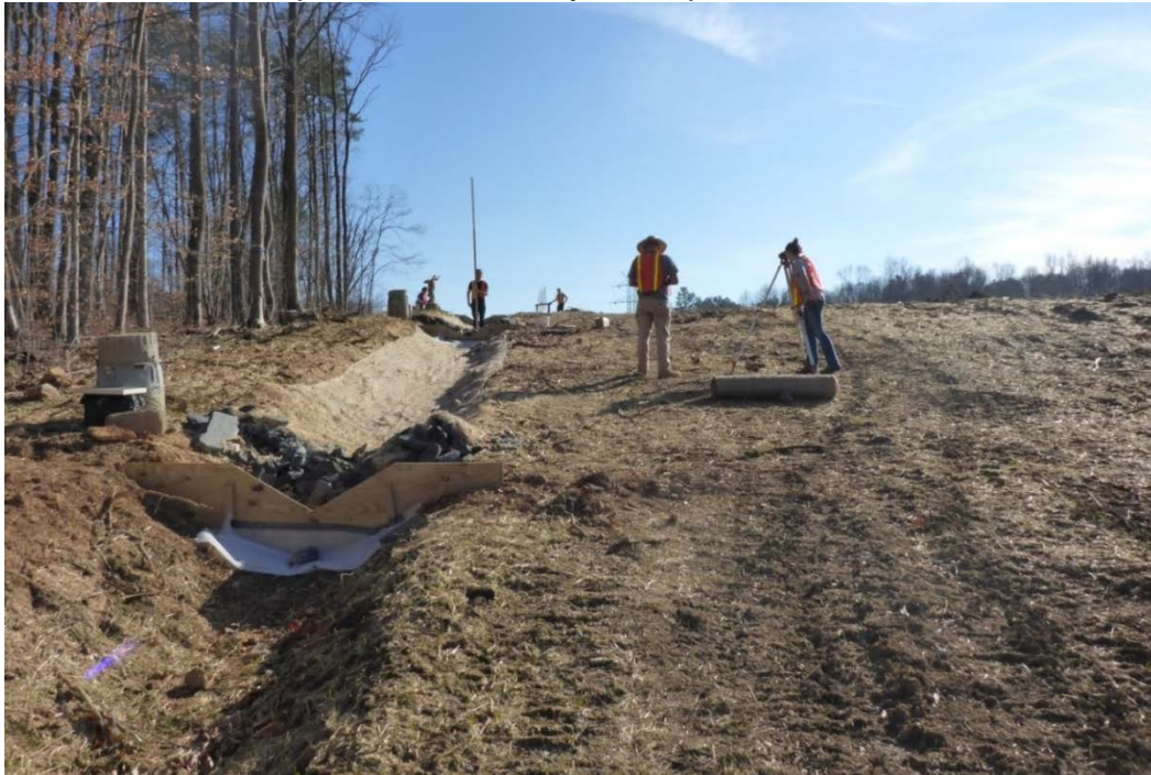
Figure 6. Measuring the slope of each ditch section. Note V-notch weir and sampler placed to measure flow and sediment loss.
