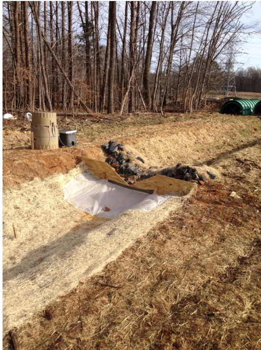
Figure 9. Automated sampler and V-notch weir for collecting water quality and quantity data.
