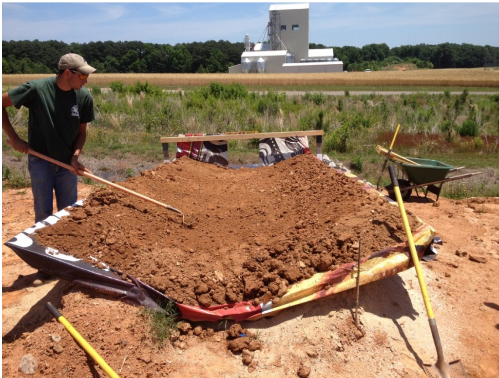
Figure 1. Spreading soil in the flume prior to packing.
