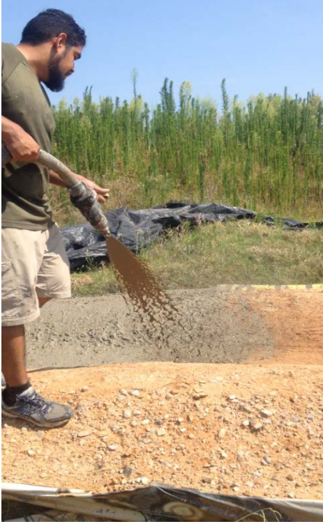
Figure 4. Posi-Shell being applied to the simulated ditch at SECREP.
