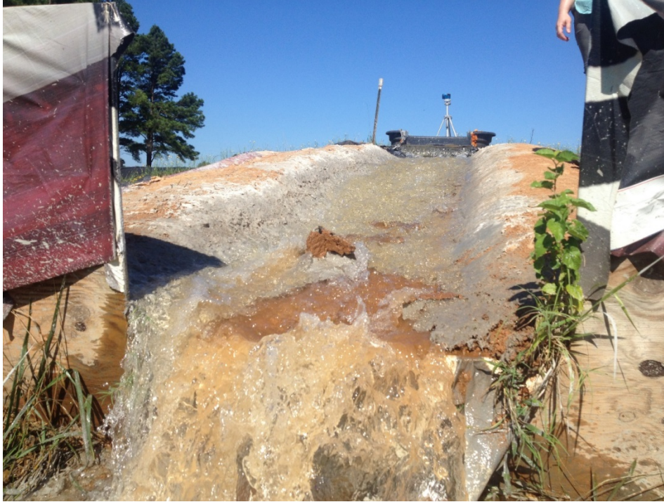
Figure 30. Failure of the Posi-Shell at the steepest (12%) slope. This may have been an artifact due to the high turbulence at the point where the liner meets the weir – notice how it started at the bottom.
