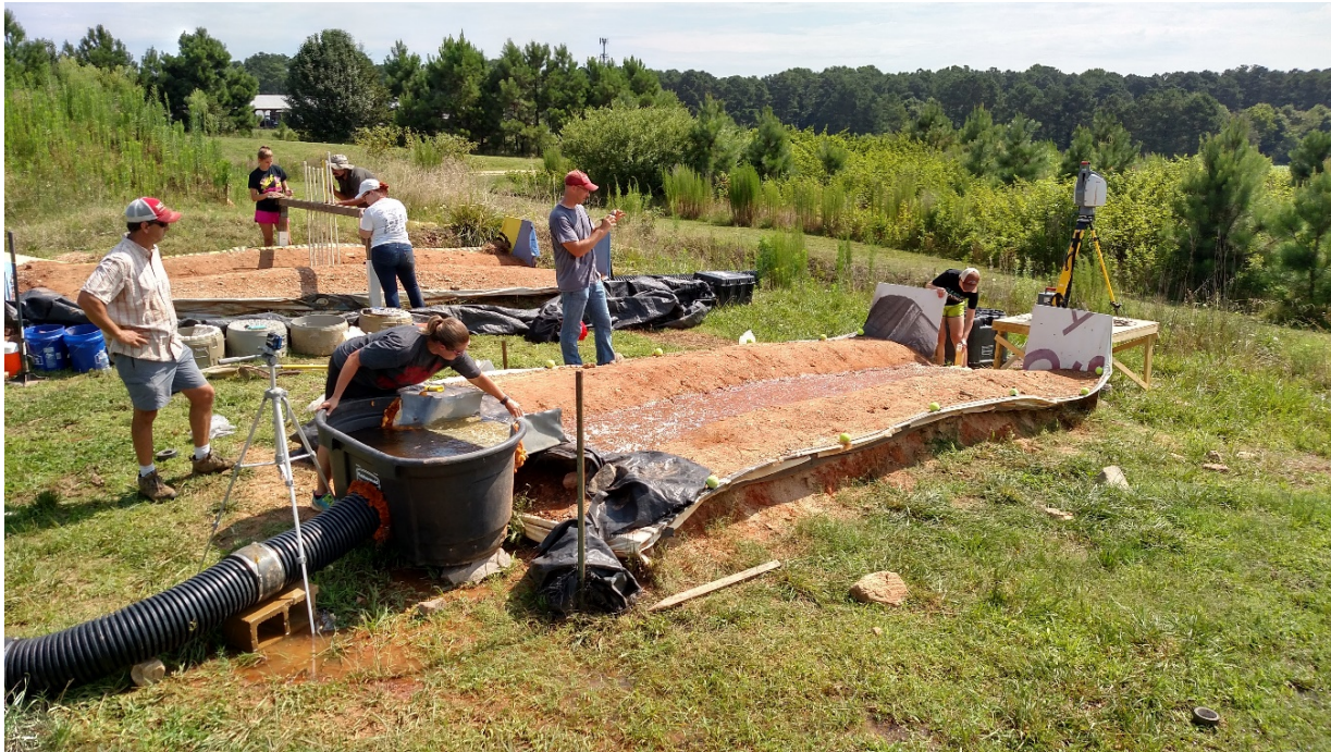
Figure 3. Measuring erosion with a pin device (background) and testing bare soil in the medium (8%) slope. Surveys were also conducted via georeferenced photographs and a LiDAR unit, shown at the end of the closer flume, for several tests. Manual collection of inlet and outlet samples is also occurring in this ditch.
