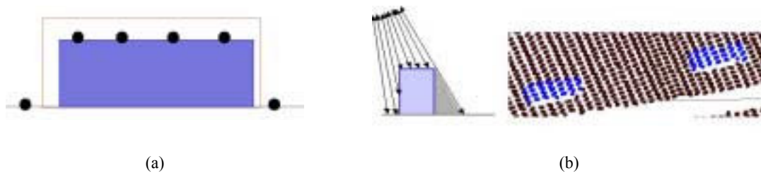
Figure 2. Limitations in accurate parameterization of LiDAR-sensed vehicles: (a) data density and footprint size, (b) shadow effect.
