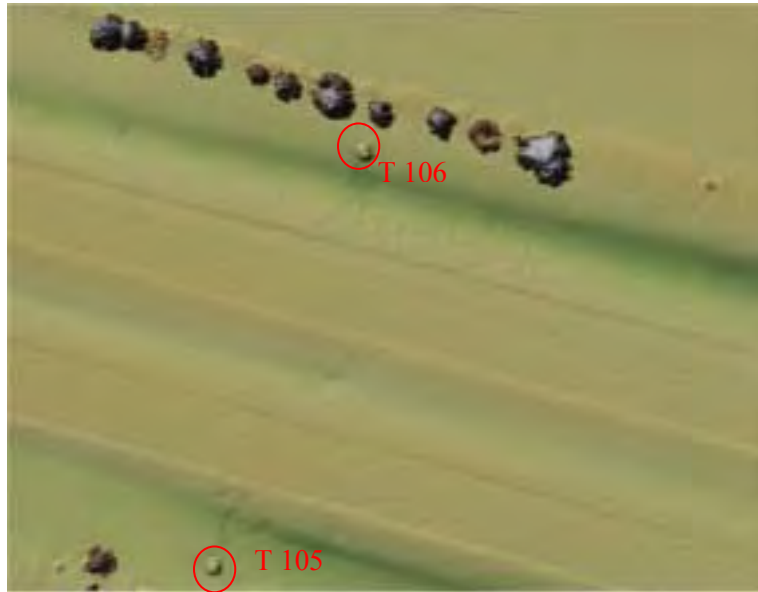
Figure 7. LiDAR targets #105 and #106 in the elevation data
