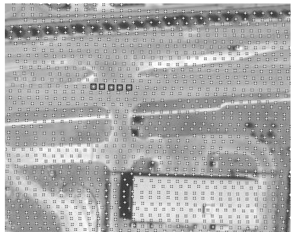
Fig. 3. LIDAR points overlaid in simultaneously acquired digital image.
