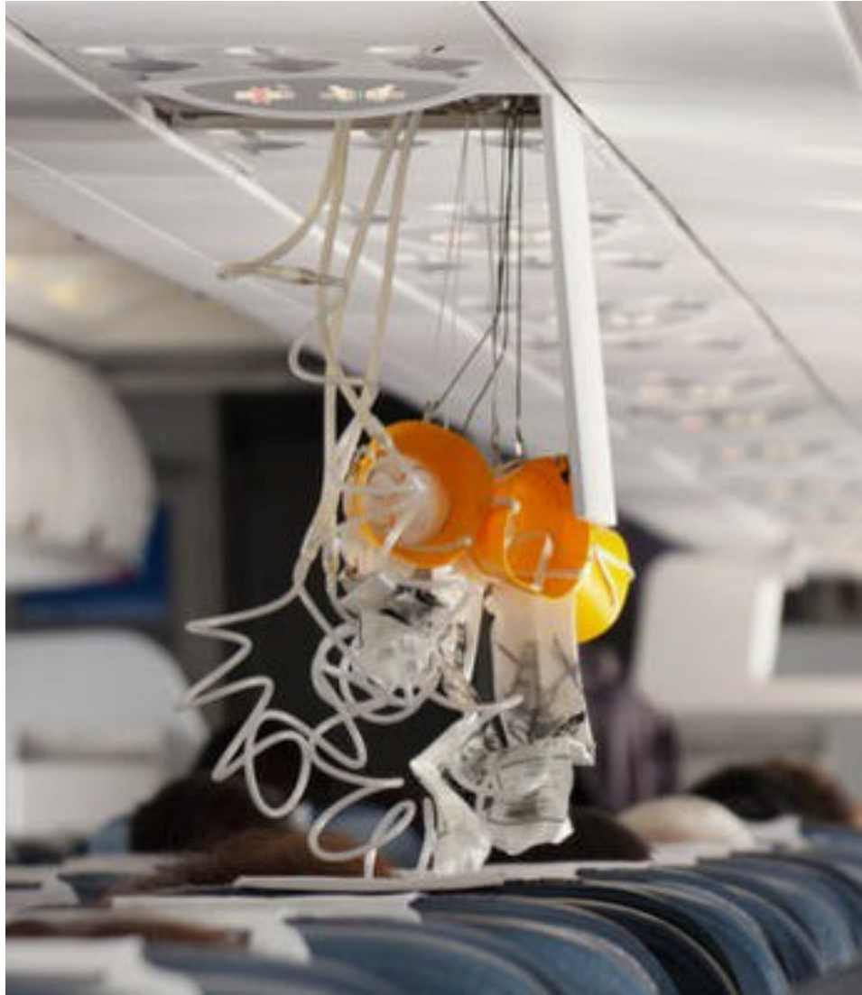
Figure 3: Deployed But Not Yet Activated Oxygen Masks
