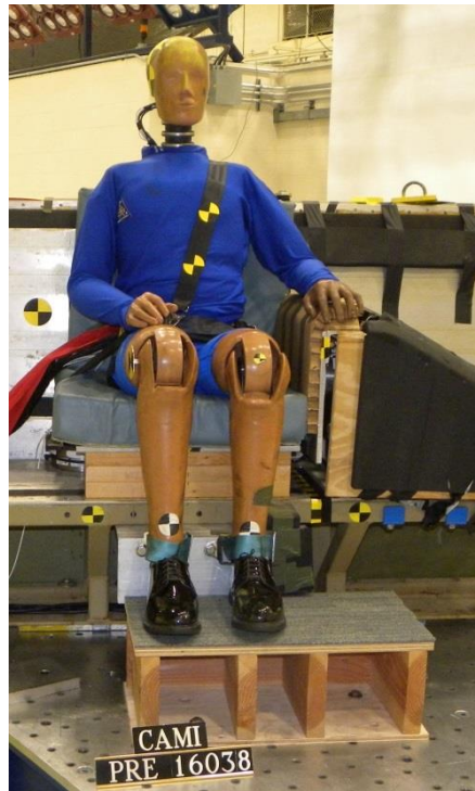
Figure 1: Oblique Seat Test with Armrest and Shoulder Harness
