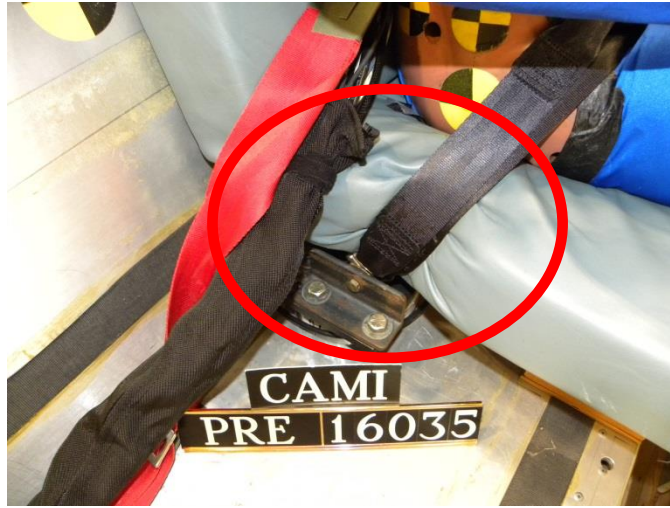
Figure 13: Compression of Seat Bottom Cushion by Lap Belt (Red Circle)
