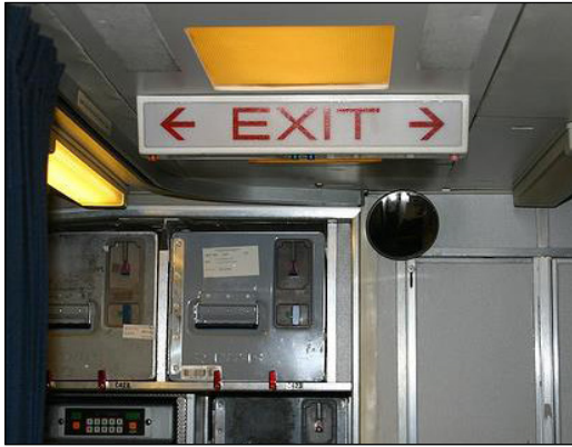
Figure 7. A traditional, text-based exit locator sign with directional indicators, which complies with the requirements of 14 CFR 25.812(b)(i).
