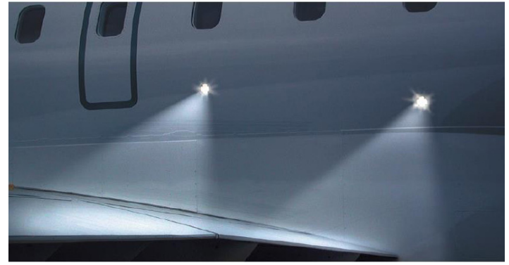
Figure 11. The illumination on the wing where an evacuee is likely to make his first step must be at least 0.03 ft-c. On the escape route on the wing, the illumination must be at least than 0.05 ft-c. (From Goodrich Interiors and Lighting Systems, 2003).
