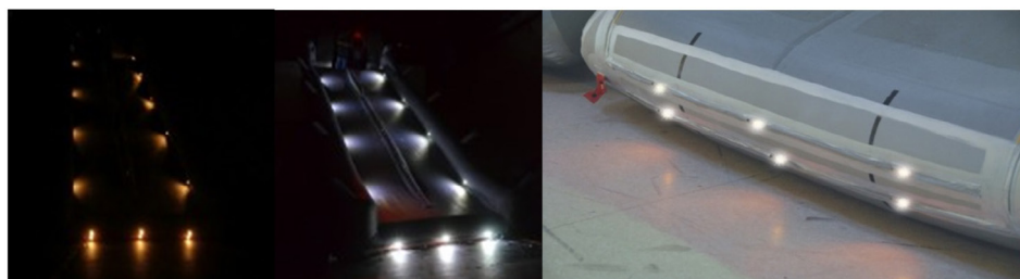
Figure 12. An example of escape slide lighting systems. Left: Incandescent lighting, Center: LED lighting, Right: Ground-illuminating LED lights at end of slide (BaseWest, http://basewest.com/slidelight_products/escape-slide-lighting ).
