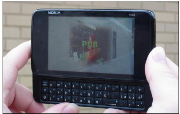
Figure 17. Example of an X ray AR navigation tool showing the destination through a building blocking physical line of sight.
