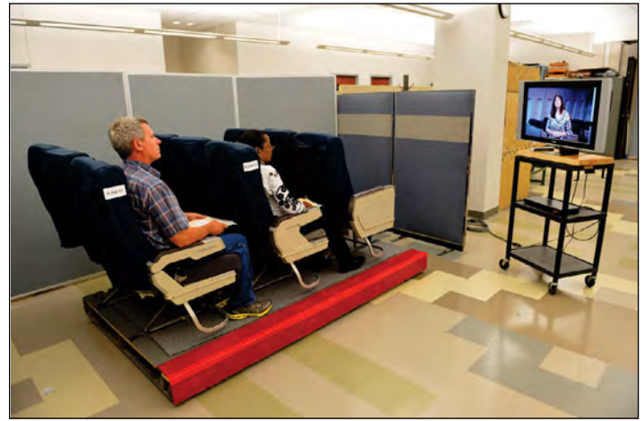
Figure 4. Study participants, seated in airplane mock-up, watch the recorded safety briefing before the life preserver donning portion of the test trial.
