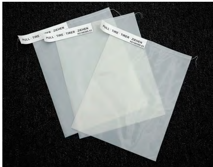
Figure J-10. Standard "tear tab" replacement package used for repacking life preservers. A single layer sheet measured 4.33 mil thick.
