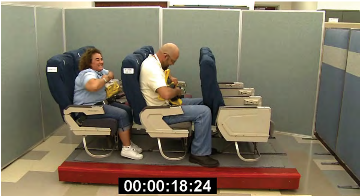
Figure 10. Female test participant struggles to open package of Life Preserver Q. She was able to remove the life preserver from the package after 37.9 seconds.
