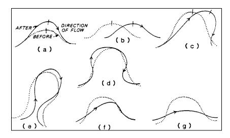
Figure 2.11. Modes of meander loop development: (a) extension, (b) translation, (c) rotation, (d) conversion to a compound loop, (e) neck cutoff by closure, (f) diagonal cutoff by chute, and (g) neck cutoff by chute (after Brice and Blodgett).<sup>(10)</sup>
