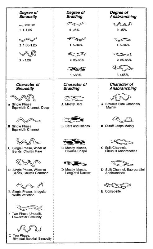
Figure 4.21. Alluvial channel pattern classification devised by Brice (after Brice 1975).<sup>(38)</sup>
