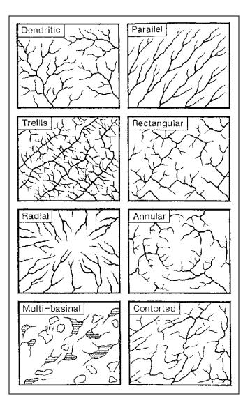
Figure 4.2. Basic drainage patterns (from Howard 1967).<sup>(35)</sup>
