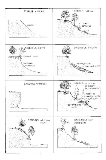
Figure 4.16. Classification and morphology of typical bank profiles.<sup>(34)</sup>
