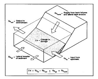
Figure B.1. Schematic representation of sediment fluxes to and from river bank basal zones.<sup>(13)</sup>
