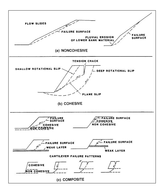
Figure 2.9. Typical bank failure surfaces: (a) noncohesive, (b) cohesive, and (c) composite (after Brown).<sup>(17)</sup>
