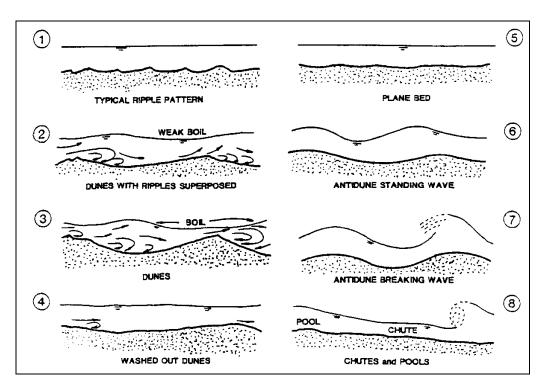
Figure 5.4(a). Forms of bed roughness in sand channels (after HDS 6).<sup>(13)</sup>
