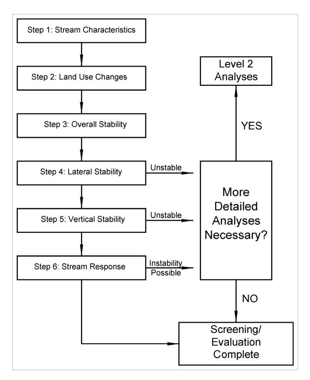
Figure 3.1. Flow chart for Level 1: Qualitative Geomorphic Analyses.
