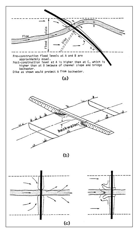
Figure 5.8. Backwater effect associated with three types of stream crossings: (a) a skewed alignment across a floodplain, (b) constriction of channel flow, and (c) constriction of overbank flow (after Neill).<sup>(68)</sup>
