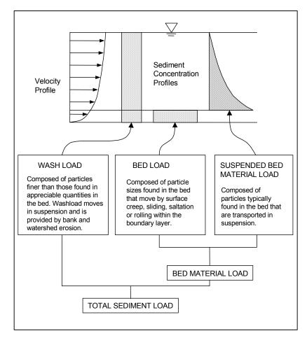
Figure 6.8. Definition of sediment load components.
