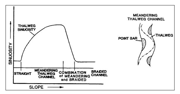
Figure 4.26. Sinuosity vs. slope with constant discharge (after HDS 6).<sup>(13)</sup>
