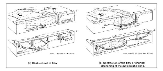
Figure 3.6. Local scour and contraction scour related hydraulic problems at bridges related to (a) obstructions to the flow or (b) contraction of the flow or channel deepening at the outside of a bend.<sup>(10,11)</sup>
