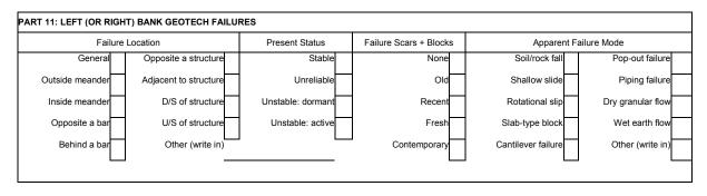
Figure 4.19. Reconnaissance sheet - left (or right) bank geotechnical failures.
