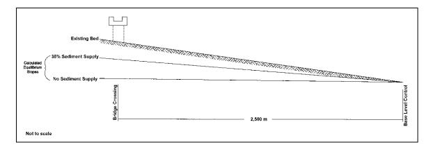
Figure E.2. Computed channel profiles from the bridge downstream to the base level control.
