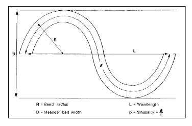
Figure 4.10. Definition of meander planform parameters.<sup>(34)</sup>
