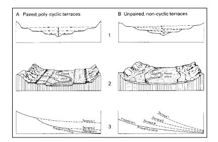
Figure 4.7. Valley cross-sections, plan view, and profiles of (A) paired, polycyclic and (B) unpaired, non-cyclic river terraces (Chorley et al. 1984).<sup>(37)</sup>
