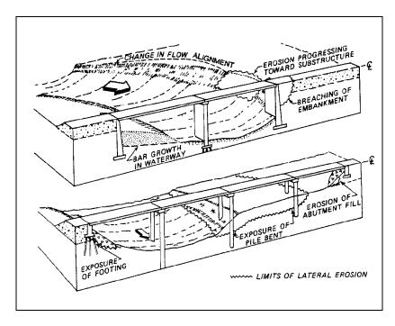
Figure 3.3. Hydraulic problems at bridges attributed to erosion at a bend or to lateral migration of the channel (after Brice and Blodgett).<sup>(10, 11)</sup>
