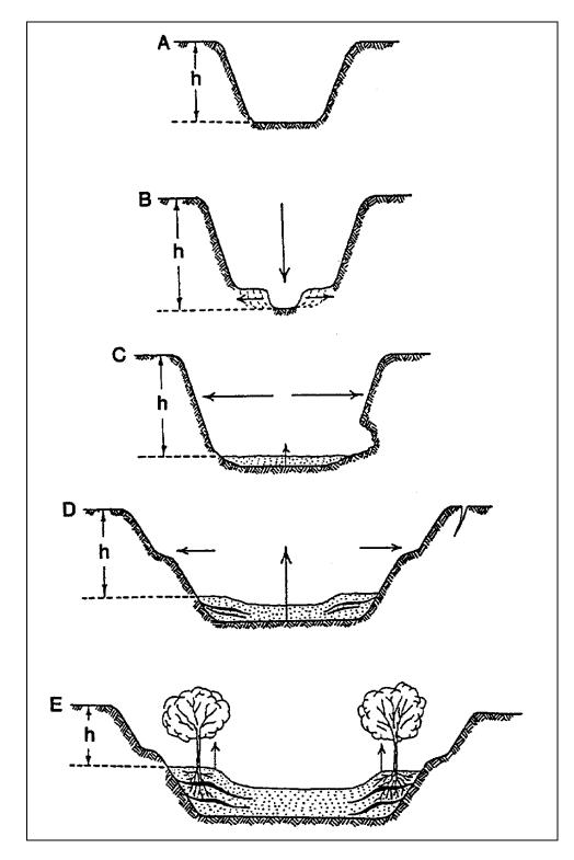
Figure 2.2. Evolution of incised channel from initial incision (A, B) and widening (C, D) to aggradation (D, E) and eventual relative stability; h is bank height.<sup>(7)</sup>
