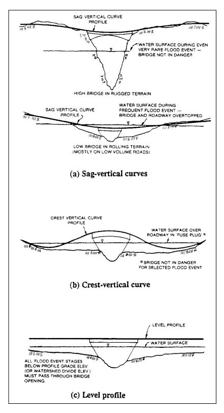
Figure 5.9. Various highway profiles: (a) sag-vertical curves, (b) crest-vertical curve, and (c) level profile.<sup>(69)</sup>
