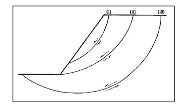
Figure B.3. Rotational slip failures in a cohesive bank: (i) slope failure, (ii) toe failure, and (iii) base failure.<sup>(2)</sup>
