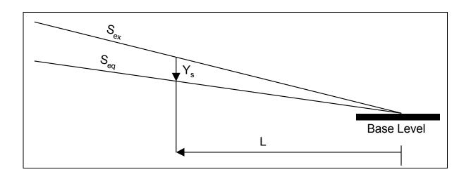
Figure 6.6. Base level control and degradation due to changes in slope.
