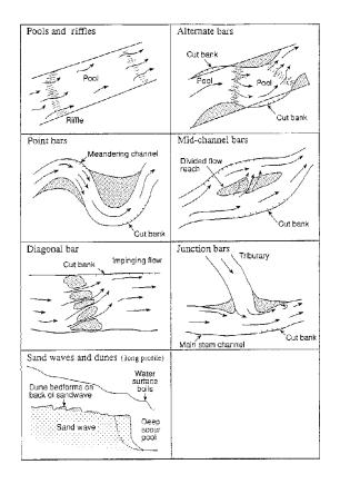
Figure 4.14. Channel bar classification and bedforms.<sup>(34)</sup>
