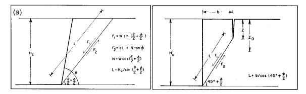
Figure B.4. Culmann analysis for (a) plane slip failure and (b) plane slip failure modified to account for tension cracking.<sup>(2)</sup>
