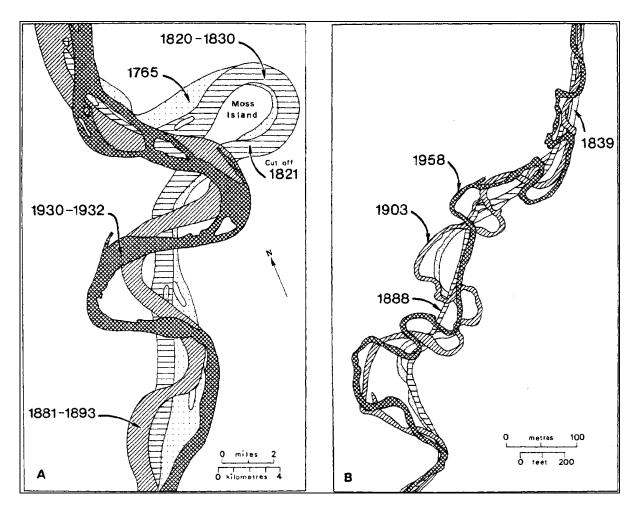
Figure 2.5. Surveys showing changes of course for two meandering rivers: (A) Mississippi River in northern Tennessee during the period 1765-1932,<sup>(3)</sup> (B) River Sid in east Devon during the period 1839-1958.<sup>(9)</sup>
