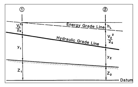
Figure 5.2. Sketch of the energy concept for open channel flow.
