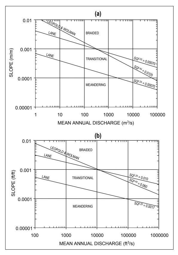
Figure 4.27a, b. Slope-discharge relationship for braiding or meandering in sand-bed streams (after Lane).<sup>(50)</sup> a = SI Units b = English Units
