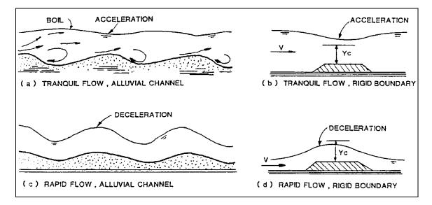
Figure 5.4(b). Relation between water surface and bed configuration (after HDS 6).<sup>(13)</sup>
