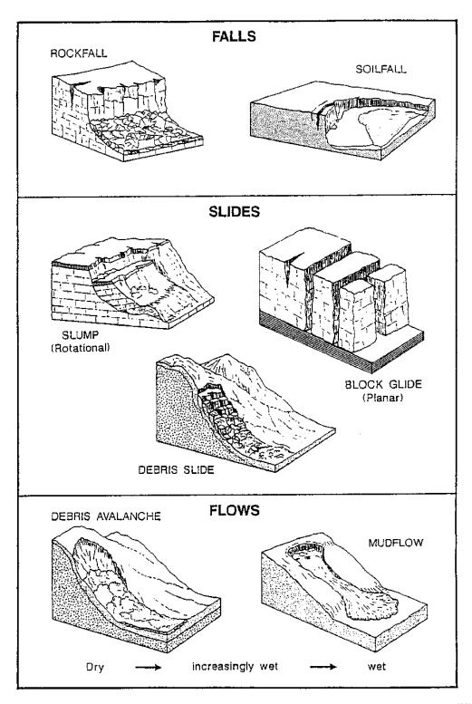
Figure 4.4. Typical valley side mass failure mechanisms (after Varnes 1958).<sup>(36)</sup>
