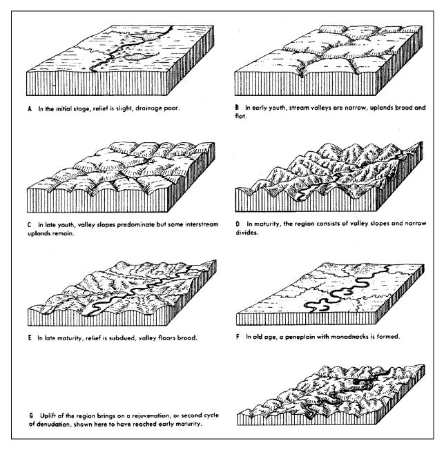
Figure 2.1. The cycle of erosion, proposed by W.M. Davis, drawn by E. Raisz.<sup>(3)</sup>
