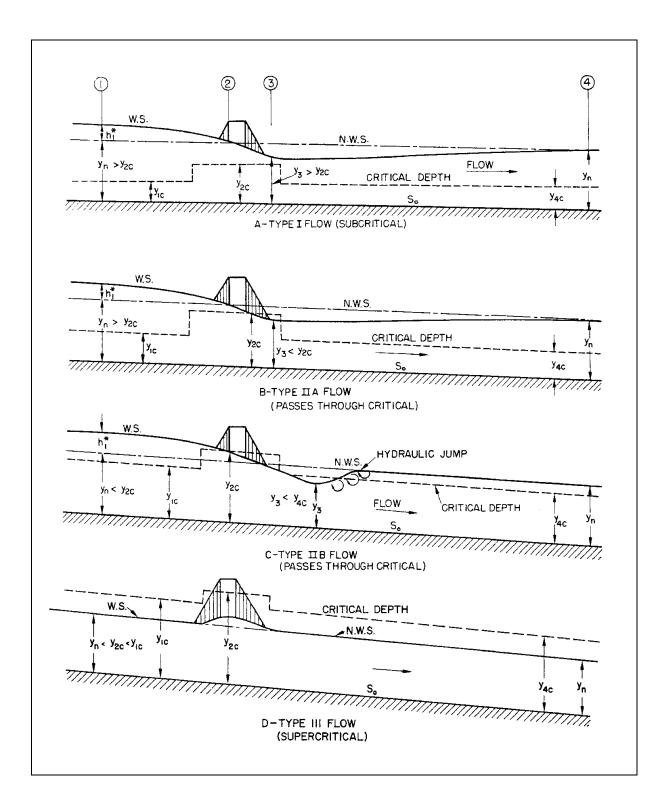
Figure 5.6. Types of water surface profiles through bridge openings (after Bradley).<sup>(66)</sup>
