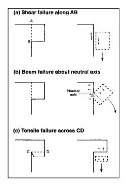
Figure B.6. Mechanisms of cantilever failure on composite banks.<sup>(22)</sup>
