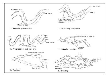
Figure 4.11. Types of lateral activity and typical associated floodplain features.<sup>(34)</sup>
