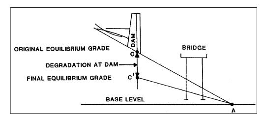
Figure 4.28. Changes in channel slope in response to a decrease in sediment supply at point C.
