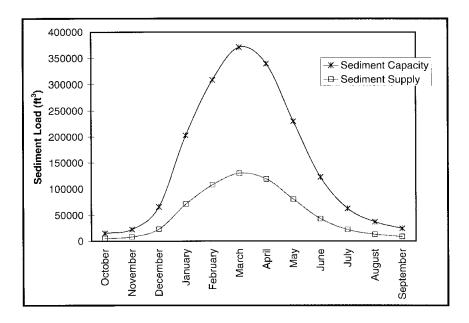
Figure E.8. Inflow (Supply) and Outflow (Capacity) Plots Corresponding to the Inflow hydrograph.
