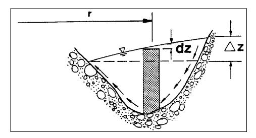
Figure 5.7. Superelevation of water surface in a bend.
