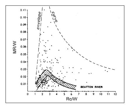
Figure 6.3. The relationship between the ratio of migration rate (MR) to channel width (W) and the ratio of radius of curvature (Rc) to width for several rivers in Canada.<sup>(94)</sup>
