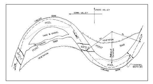
Figure 2.10. Plan view of a meandering stream.
