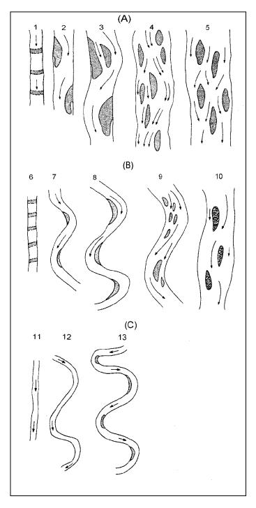
Increasing Valley Slope Increasing Stream Power Increasing Sediment Load
