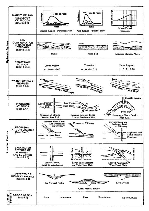
Figure 5.3. Hydraulic, location, and design factors that affect stream stability.
