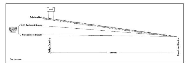
Figure E.6. Computed channel profiles from the bridge downstream to the base level control.
