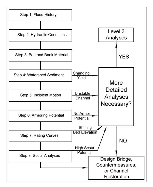
Figure 3.4. Flow chart for Level 2: Basic Engineering Analyses.
