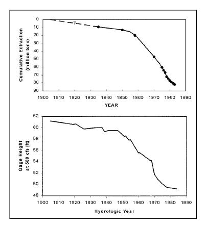
Figure 3.5. Specific gage data for Cache Creek, California.
