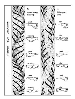
Figure 6.1. Models of flow structure and associated bed forms in straight alluvial channels:<sup>(73)</sup> (A) Einstein and Shen's<sup>(74)</sup> model of twin periodically reversing, surface-convergent helical cells, (B) Thompson's<sup>(78)</sup> model of surface-convergent flow produced by interactions between the flow and a mobile bed, creating riffle-pool units of alternate asymmetry. Black lines indicate surface currents, and white lines represent near-bed currents.
