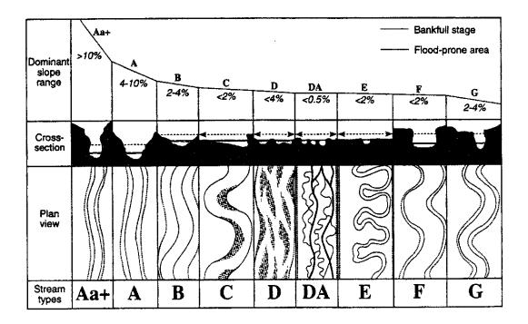
Figure 4.25. Longitudinal, cross-sectional, and planform views of major stream types in Rosgen's method (modified from Rosgen 1994<sup>(40)</sup> by Thorne<sup>(44)</sup>).
