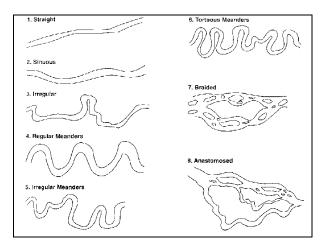
Figure 4.9. Guide to classification of river channel planform pattern.<sup>(34)</sup>
