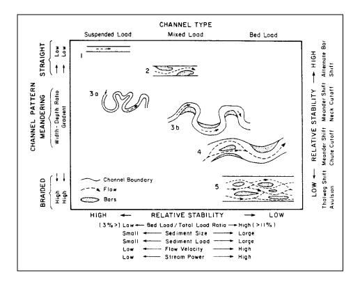
Figure 3.2. Channel classification and relative stability as hydraulic factors are varied (after Shen et al.).<sup>(16)</sup>
