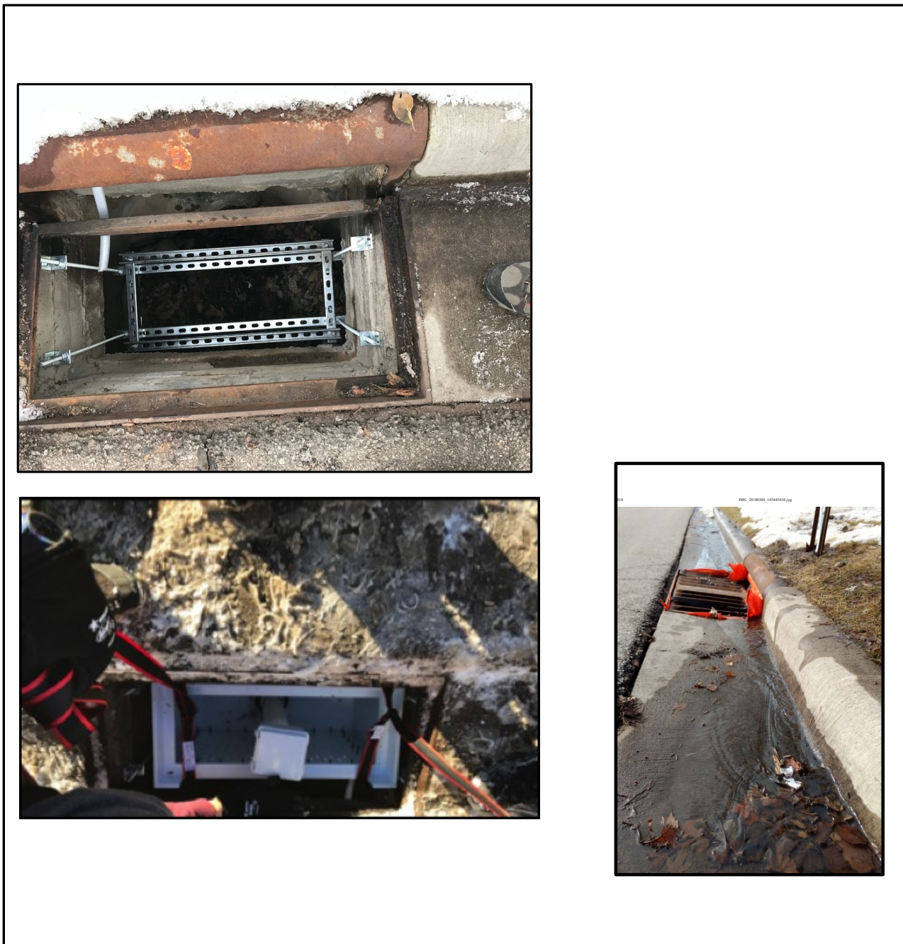
Figure 2.3: Top left: metal support frame for sampler. Bottom left sampler being lowered onto frame. Bottom right: sampler in place, with “Dandy” bag to filter runoff.
