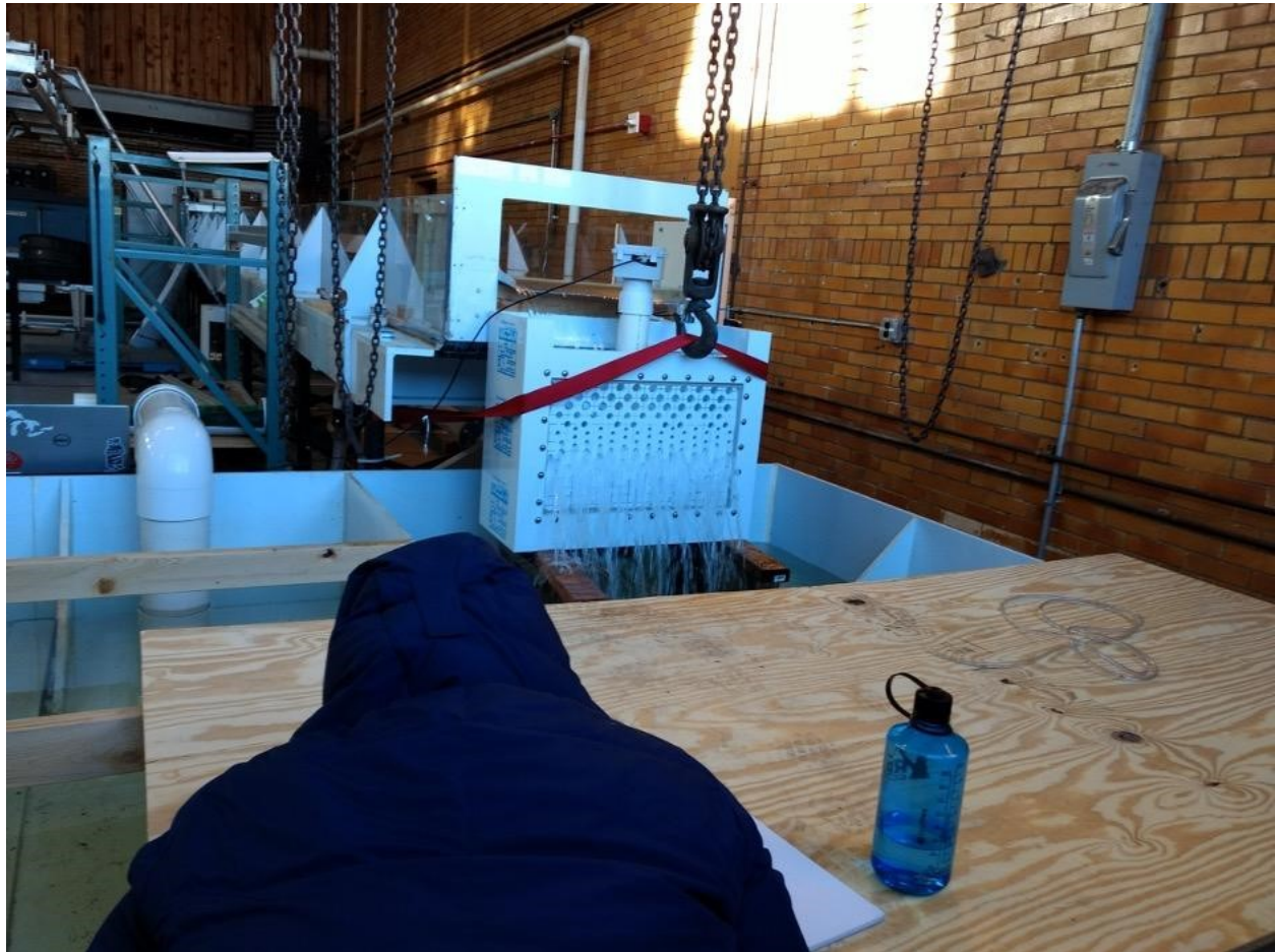
Figure 2.1: Meltwater sampler being calibrated in the lab flume in our department.
