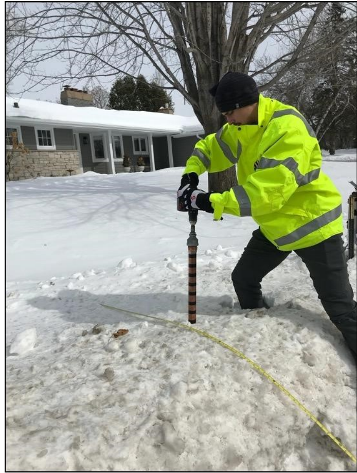
Figure 2.6: Using the snow coring device in the field.
