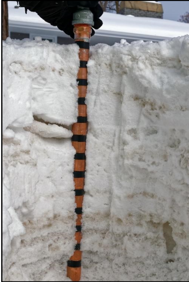
Figure 2.5: Snow coring device used in year 2.
