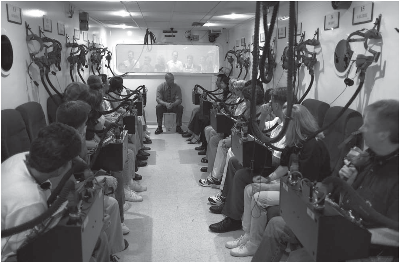
Figure 1. The Civil Aerospace Medical Institute low-pressure altitude training chamber in operation with students and an instructor inside.
