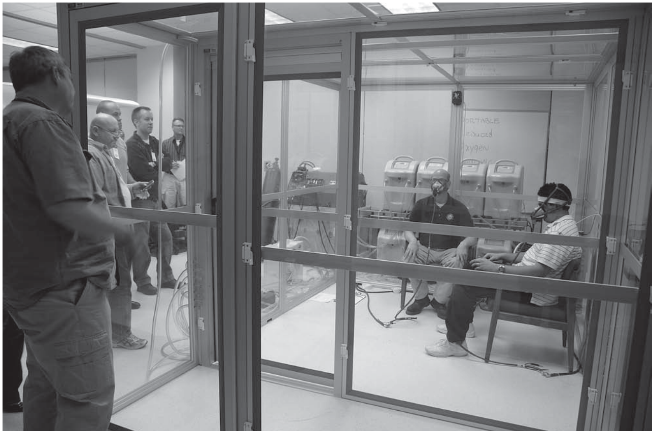
Figure 2. The Portable Reduced Oxygen Training Enclosure under test conditions.
