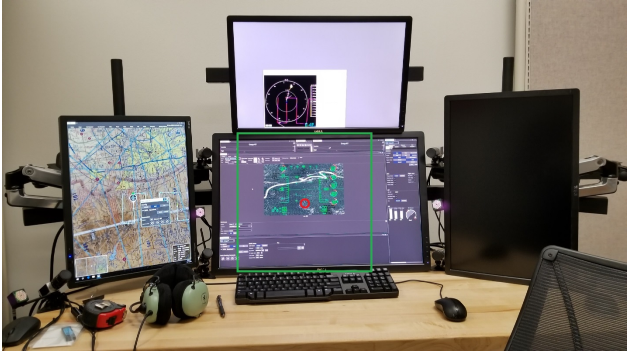
Figure 1. Vigilant Spirit control station with the traffic display on top. The design eye point is shown as a red circle. The green box depicts the primary field-of-view around the design eye point.
