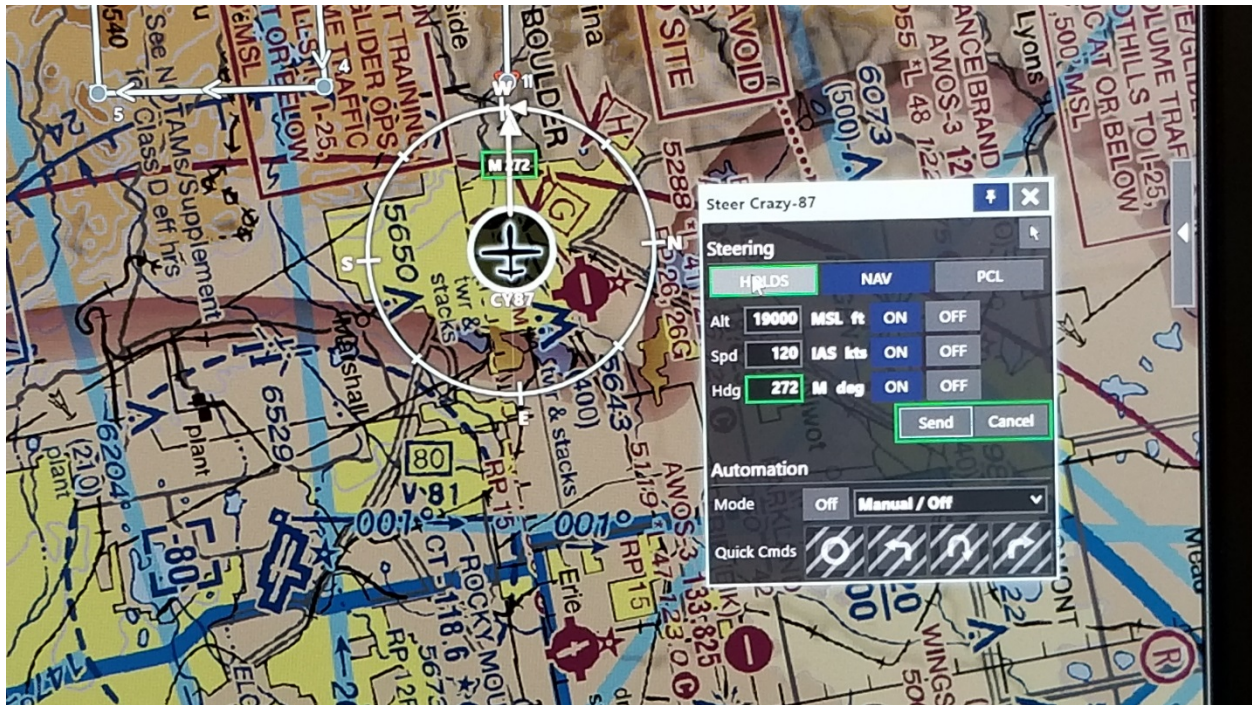
Figure 5. Steering box for sending maneuver commands to the aircraft.
