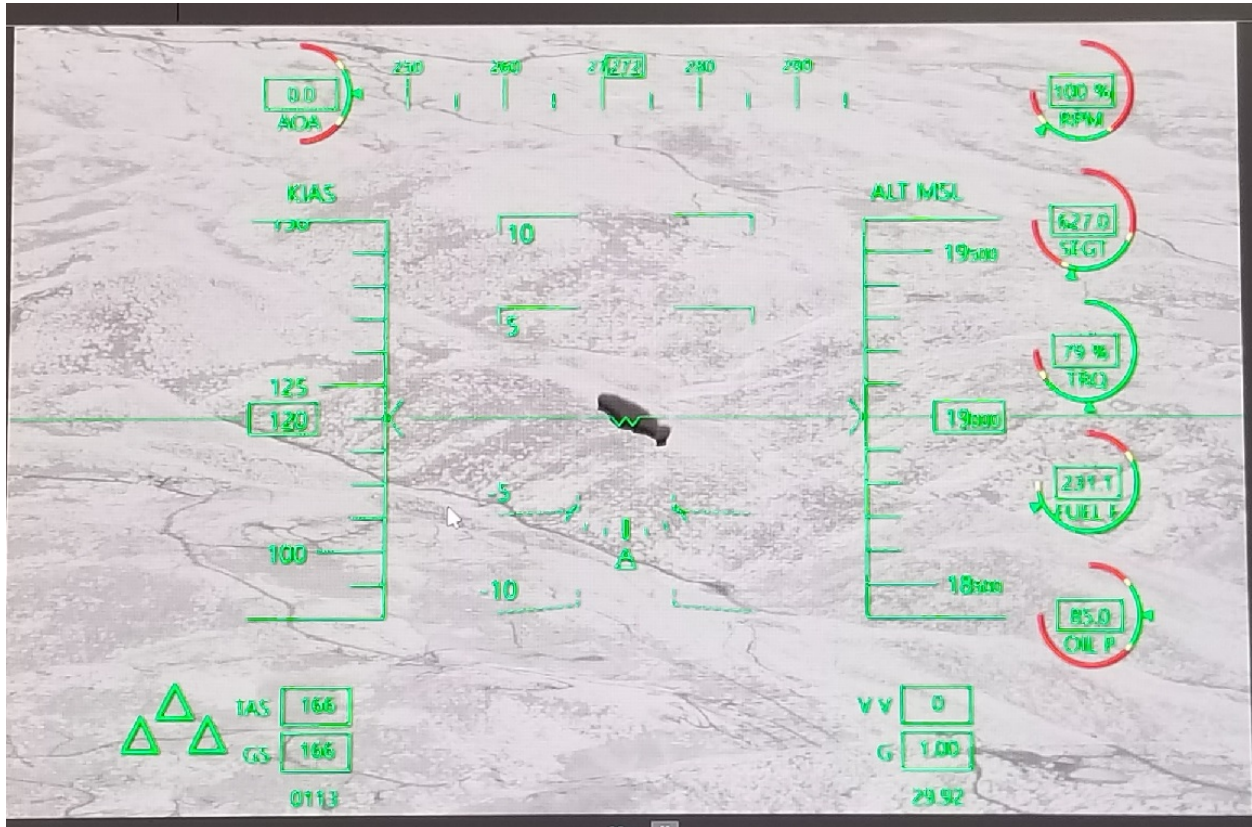
Figure 7. View of a hot spot using the Infrared (IR) setting with Black-Hot mode.
