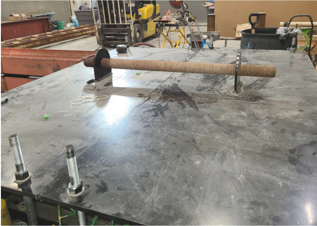
Figure 4.11 A rigid steel rod that runs through the reaction plate to minimize any differential deformation of the plate.
