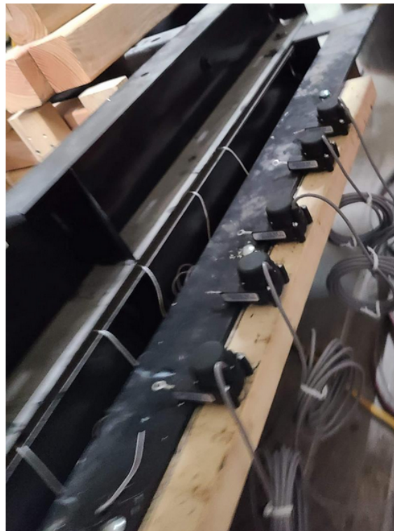
Figure 4.8 LVDTs (telltales) attached to the rear portion of the test box.
