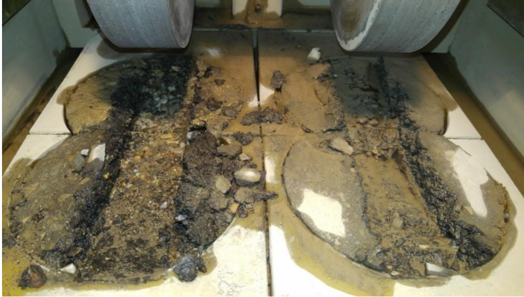
Figure 8 – Post Test Picture of Wet Hamburg Wheel Tracking for Tucson Airport Surface Course
