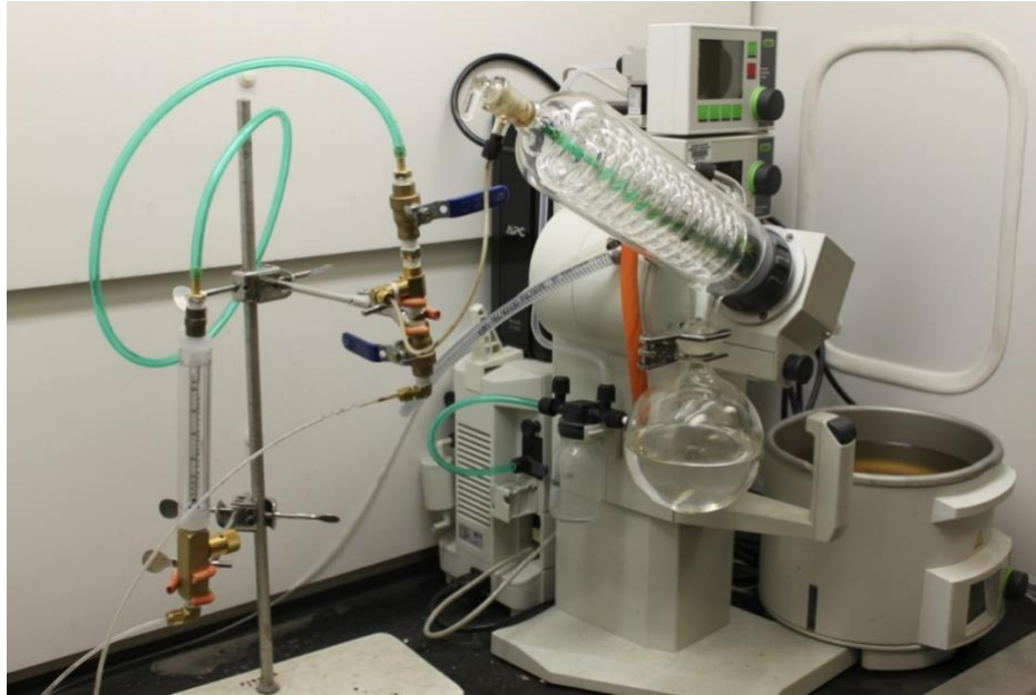
Figure 17 – Asphalt Binder Recovery Equipment at Rutgers University
