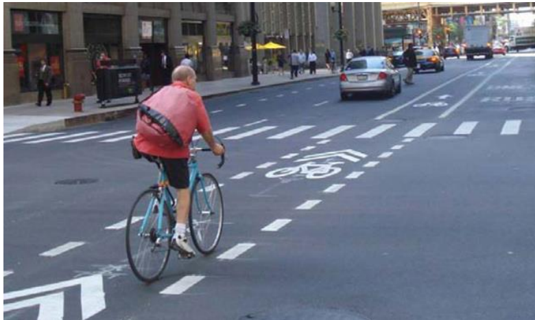
Figure 2.20: Intersection Crossing Marking with Dotted Lines and Shared Lane Marking (source: NACTO )
