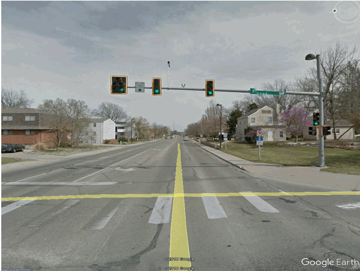
Figure 3.3: Google Earth being used to identify the type of left turn signal, the presence of RTOR, and lighting in one approach of a 4SG intersection
