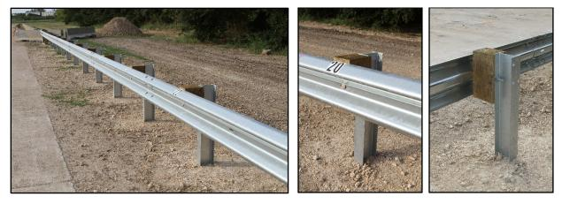
Figure 2.4. MGS Strong Post System prior to Testing.
