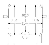
'Lateral area across the cab from driver's side kickpanel to passenger's side kickpanel.
