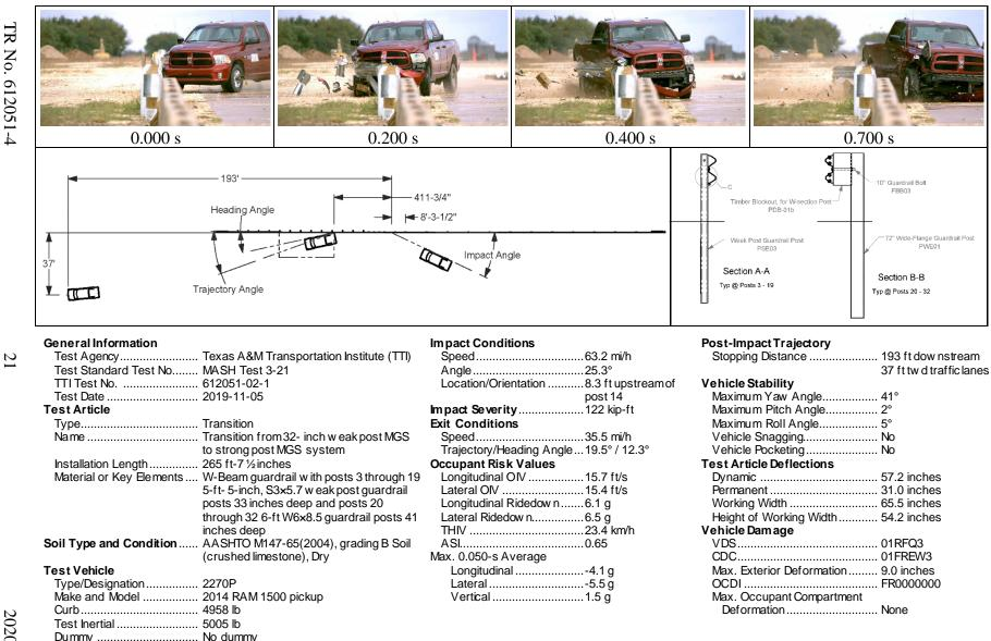
Figure 5.10. Summary of Results for MASH Test 3-21 on Guardrail Transition from 32-inch Tall MGS Weak Post System to the MGS Strong Post System.
