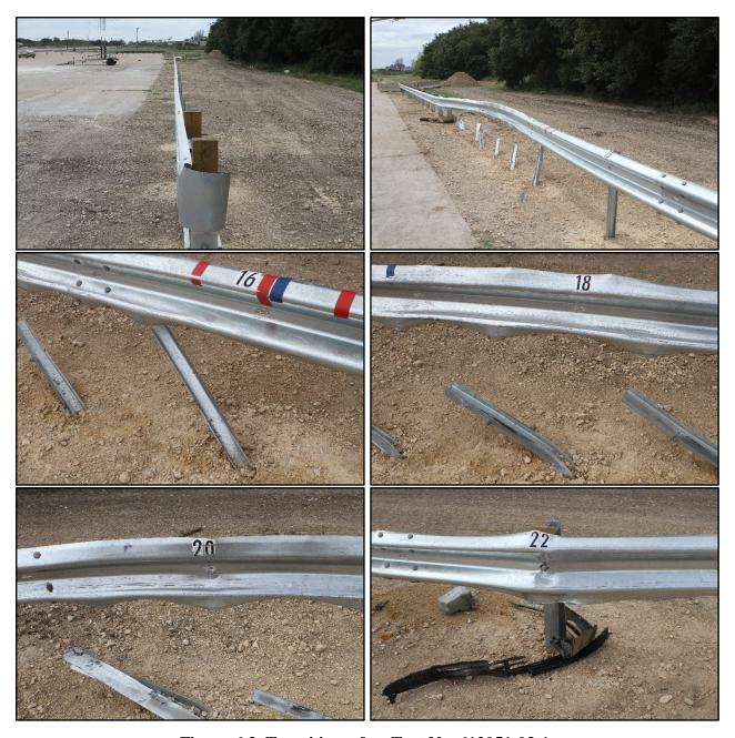
Figure 6.3. Transition after Test No. 612051-03-1.
