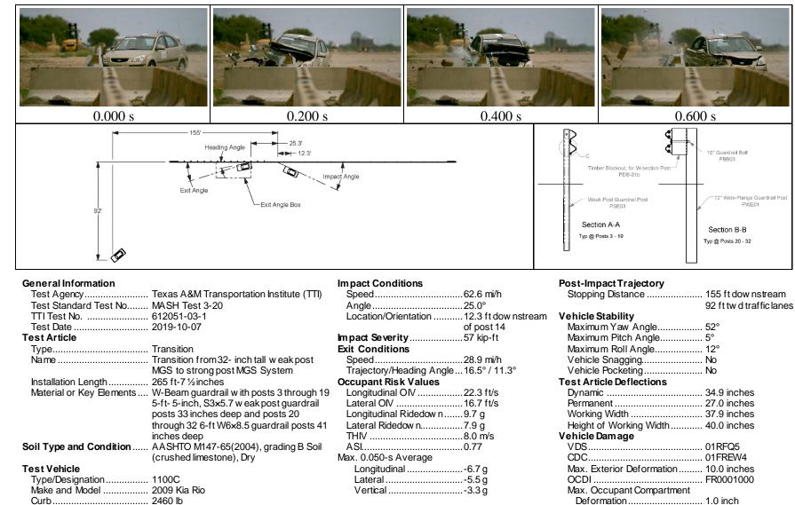
Figure 6.6. Summary of Results for MASH Test 3-20 on Guardrail Transition from 32-inch tall MGS Weak Post System to the MGS Strong Post System.
