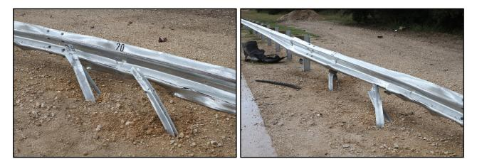
Figure 5.6. Posts 19 through 25 after Test No. 612051-02-1.
