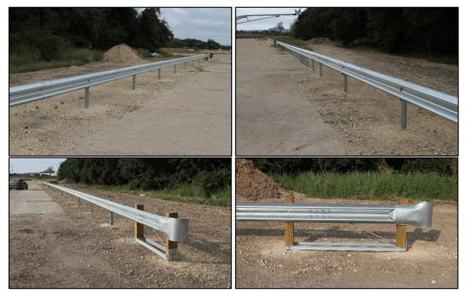
Figure 2.2. Guardrail Transition from 32-inch Tall MGS Weak Post System to MGS Strong Post System prior to Testing.
