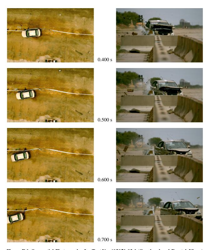
Figure E.1. Sequential Photographs for Test No. 612051-03-1 (Overhead and Frontal Views) (Continued).
