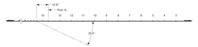
Figure 3.1. Target CIP for MASH Test 3-20 on Guardrail Transition from 32-inch tall MGS Weak Post Guardrail System to MGS Strong Post System.
