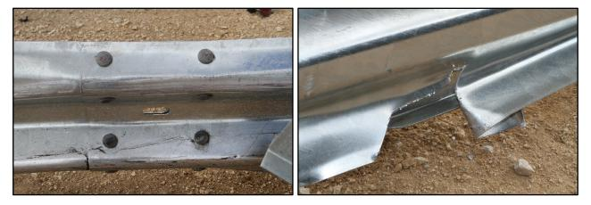
Figure 5.7. Partial Tear of Rail Element after Test No. 612051-02-1.
