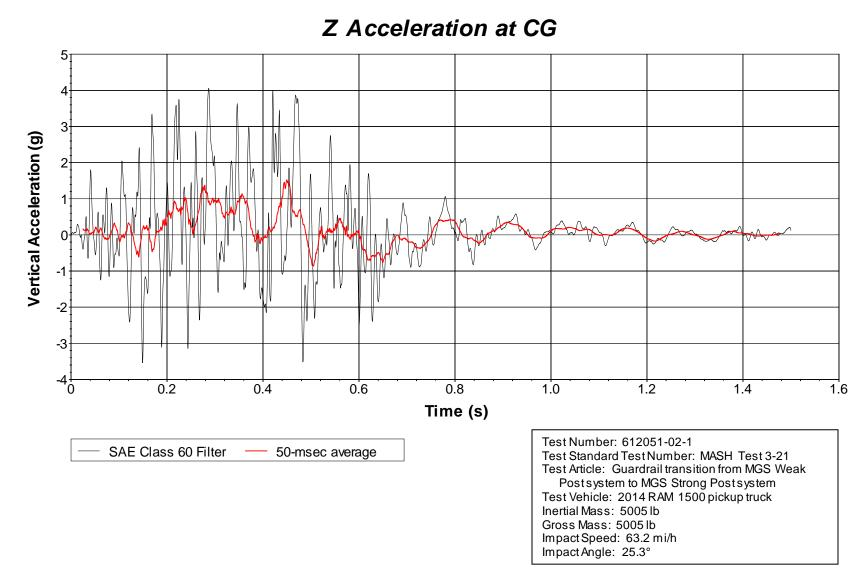
Figure D.6. Vehicle Vertical Accelerometer Trace for Test No. 612051-02-1 (Accelerometer Located at Center of Gravity).
