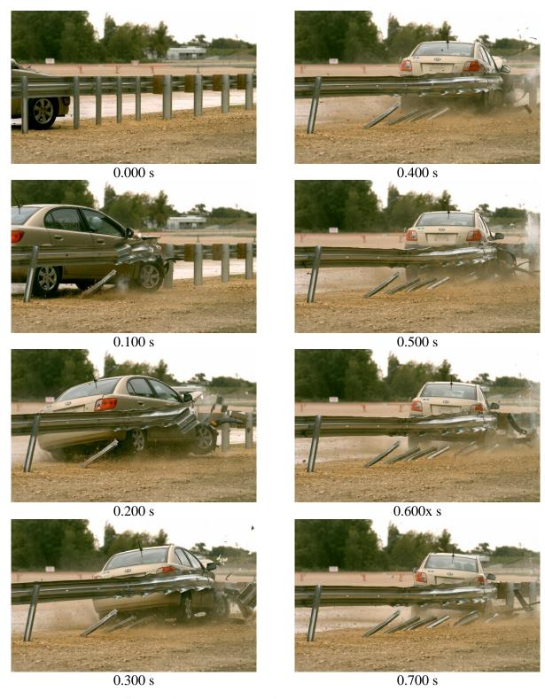
Figure E.2. Sequential Photographs for Test No. 612051-03-1 (Rear View).
