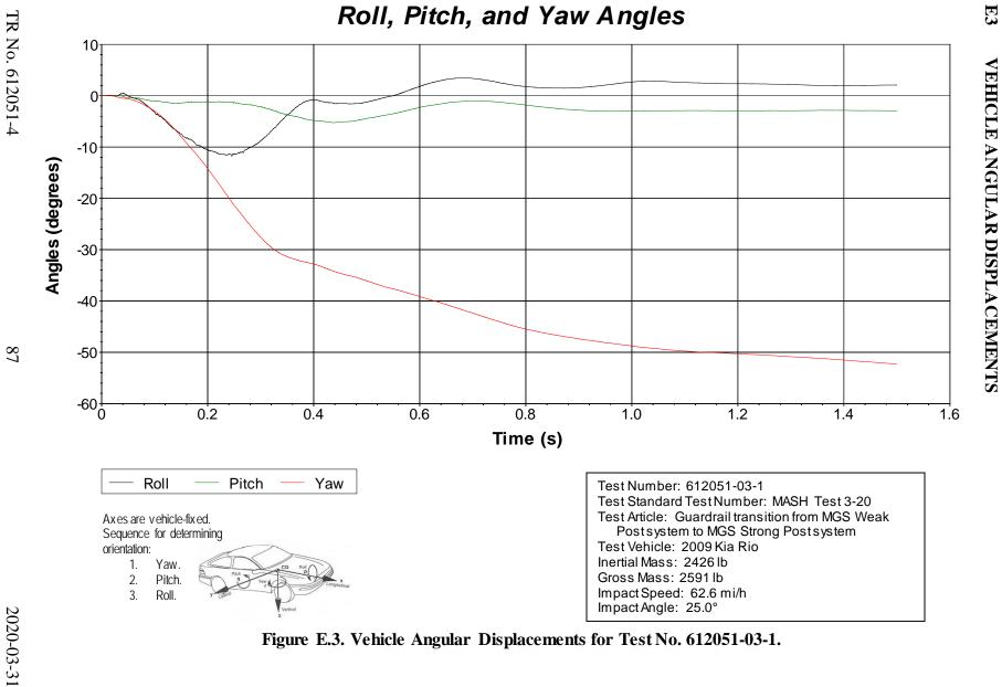
Figure E.3. Vehicle Angular Displacements for Test No. 612051-03-1.
