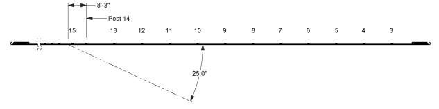
Figure 3.2. Target CIP for *MASH* Test 3-21 on Guardrail Transition from 32-inch tall MGS Weak Post System to MGS Strong Post System.
