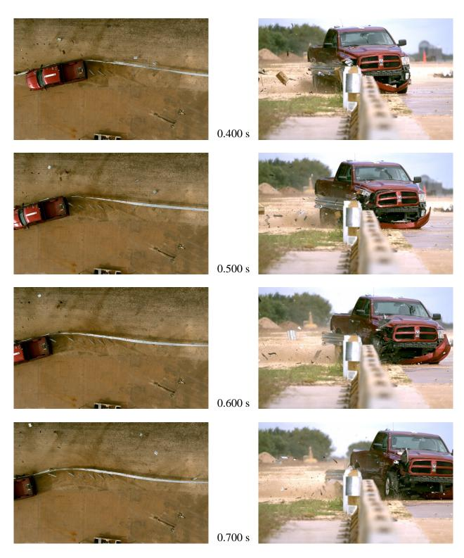
Figure D.1. Sequential Photographs for Test No. 612051-02-1 (Overhead and Frontal Views) (Continued).
