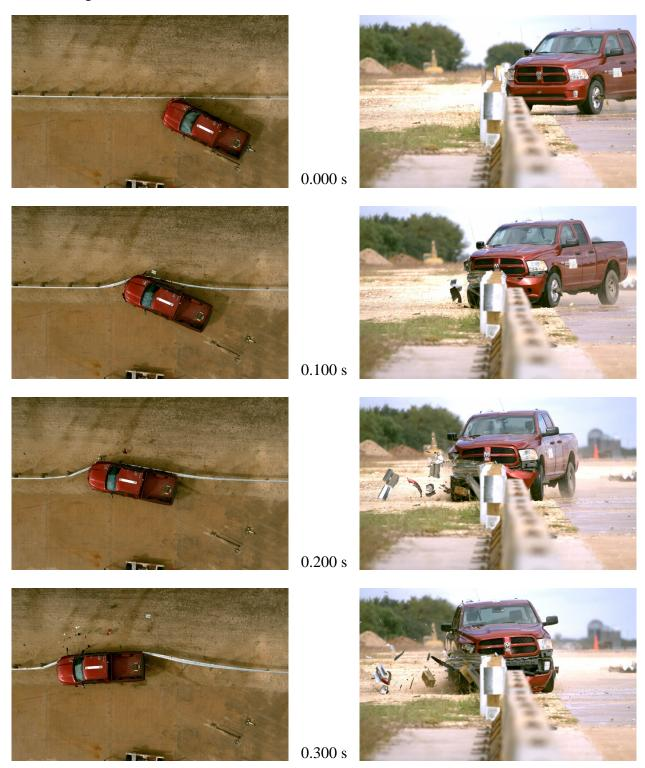
Figure D.1. Sequential Photographs for Test No. 612051-02-1 (Overhead and Frontal Views).
