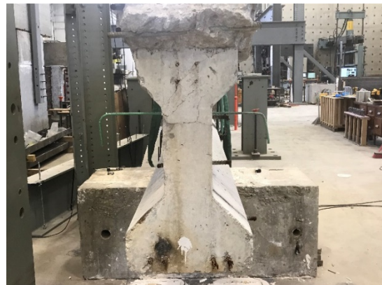
(j) Completed Installation of No. 3 Bar
