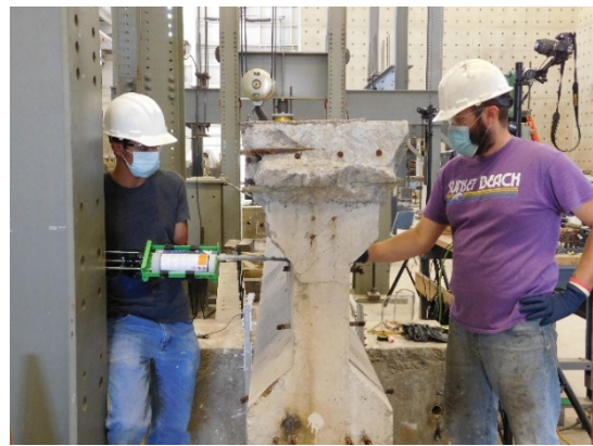
(b) Injecting Hole with Epoxy
