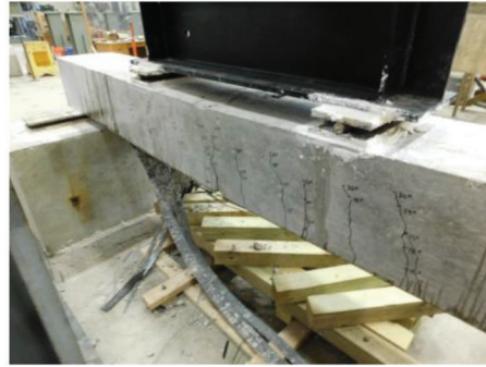
(c) Crack Pattern
