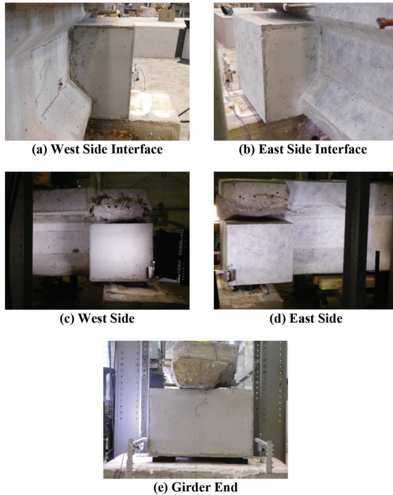
Figure 5.18 Supplemental diaphragm specimen prior to testing.
