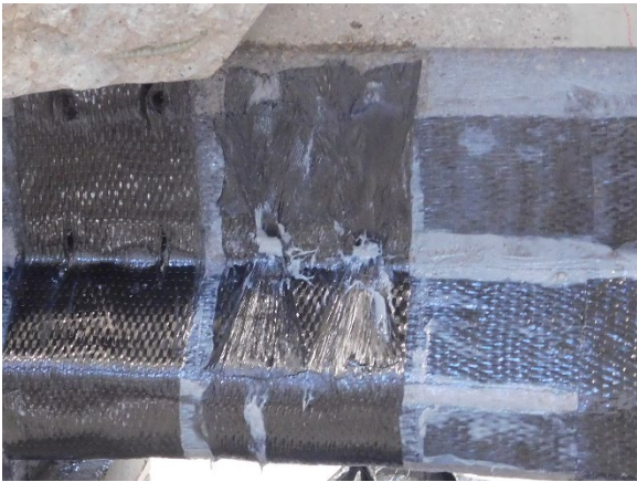
(e) Fanned-Out Anchors
