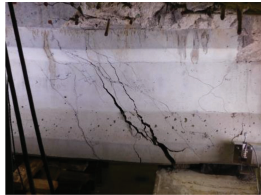
Figure 4.6 Control specimen after failure.
