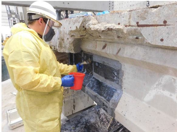
(f) Saturating Anchors
