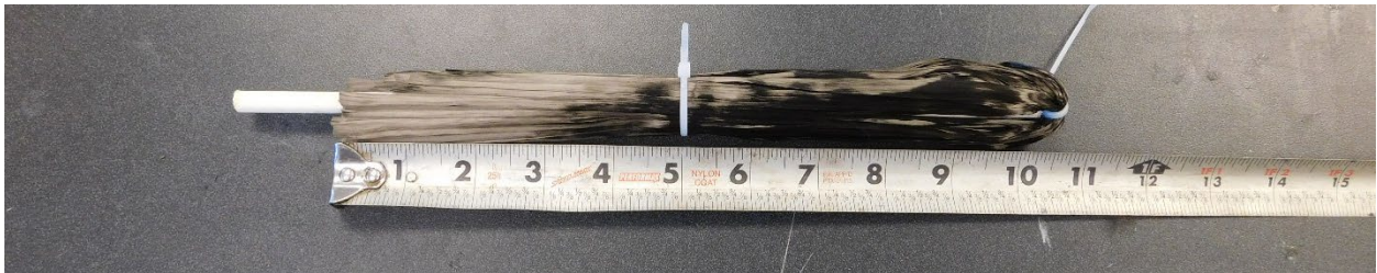
Figure E.14 Assembled FRP spike anchor for bottom flange installation.
