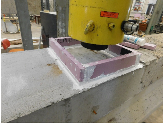
(a) Closed-Cell Polystyrene Formwork
