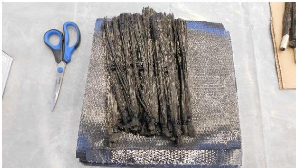
(c) Cut FRP Anchors
