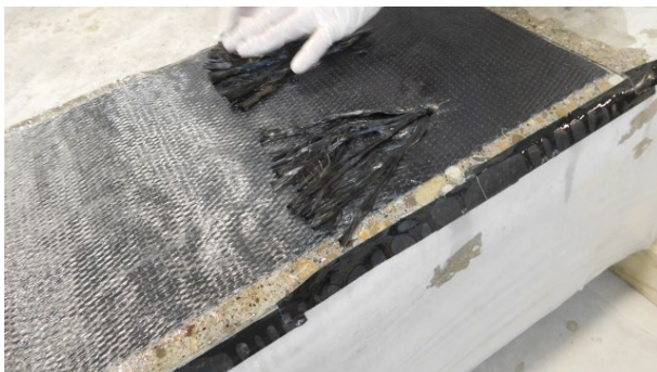
(e) Fanned-Out Anchors
