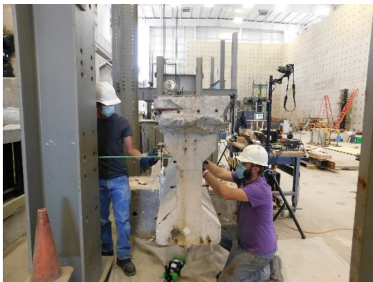
(c) Inserting No. 3 Bar Through Web
