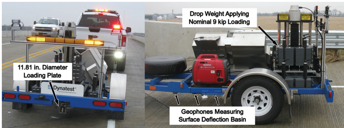
Figure 4.2 Dynatest falling weight deflectometer test setup.
