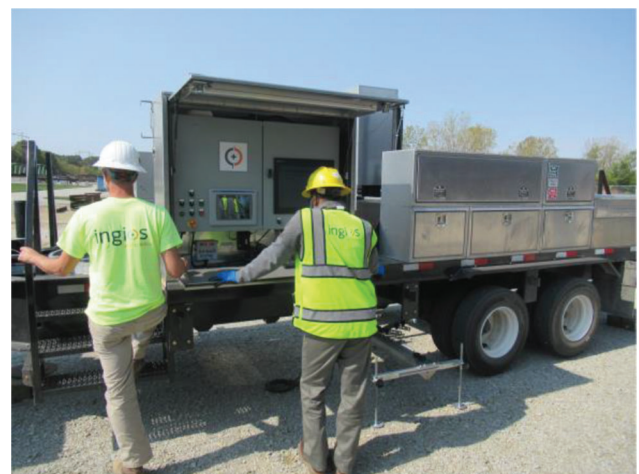
Figure 6.1 Overview of automated plate load test (APLT).
