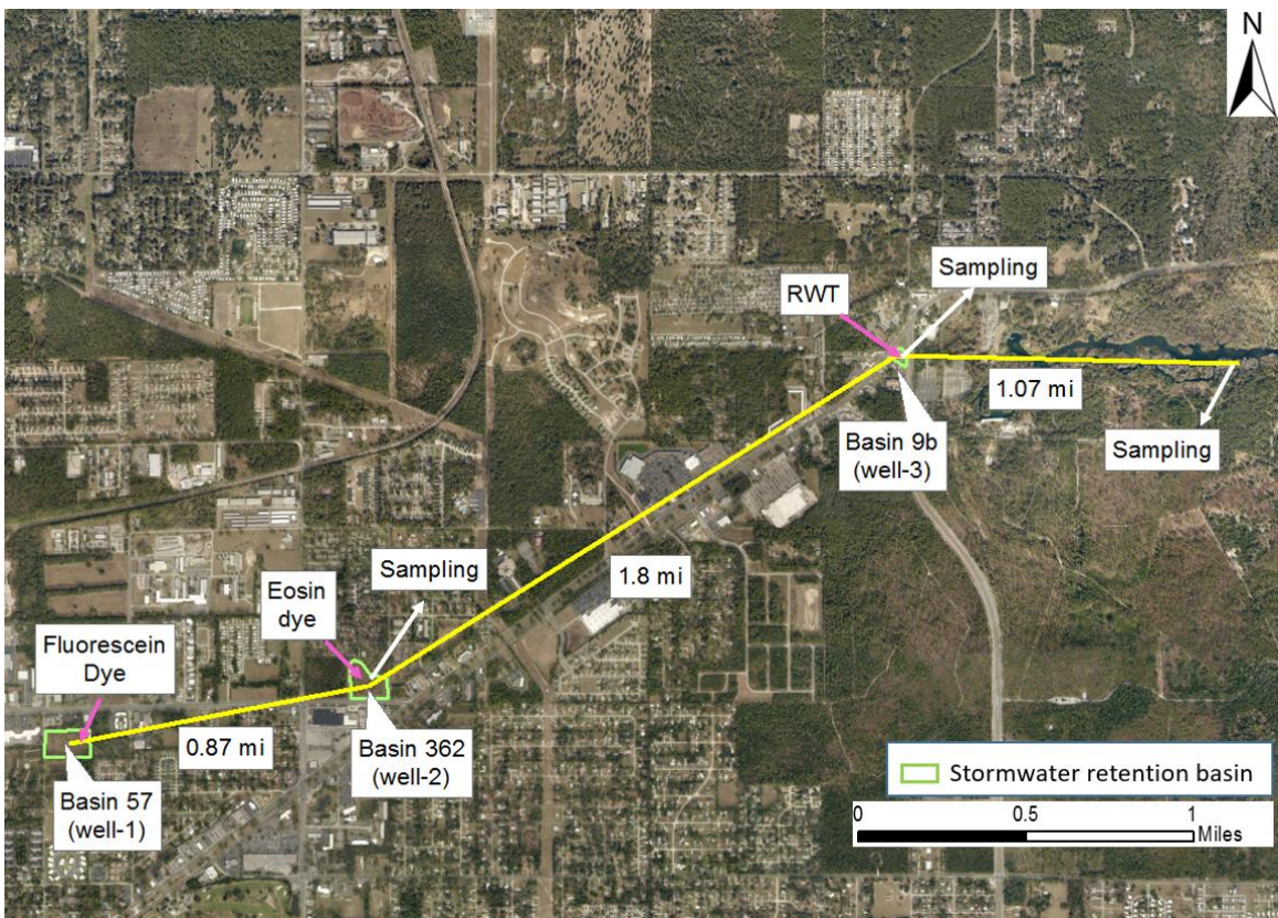
Figure 5.1. Well and spring sampling locations and dye injections to support development of the groundwater model.
