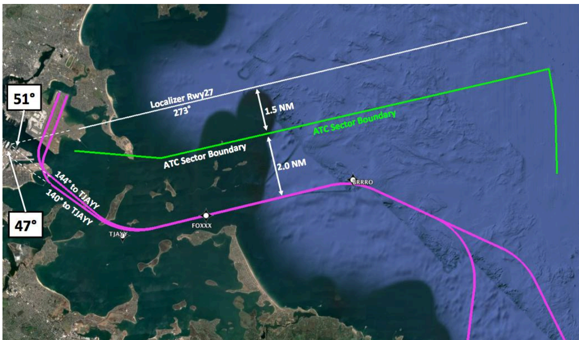
Figure 17. Baseline procedure definitions for RNAV SIDs from Runway 22L and 22R (magenta) shown with ILS Localizer to Runway 27 (white) and the air traffic control sector boundary (green)
