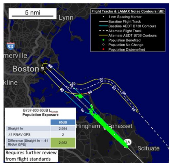
Figure 14. Horizontal Profile Modification RNAV GPS Noise Benefits for Boeing 737-800
