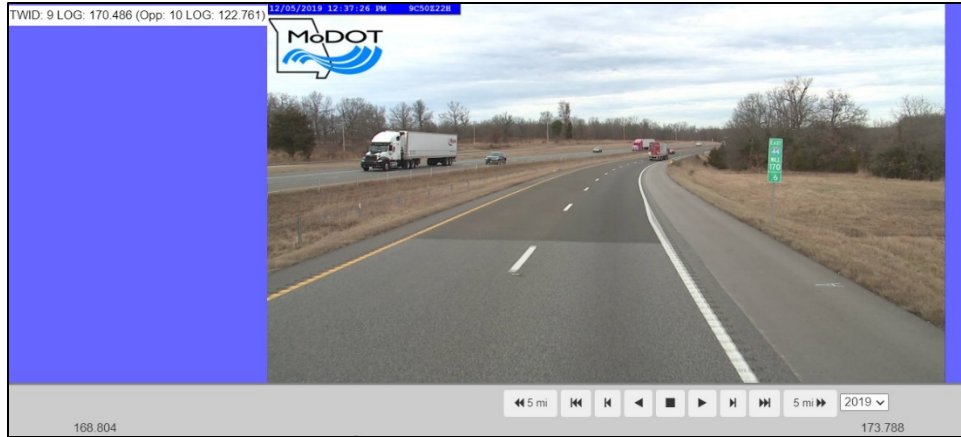
Figure 4.1. Example of ARAN viewer used to confirm HFST locations and log miles for use in analysis. (Phelps County I-44, near Powellville)
