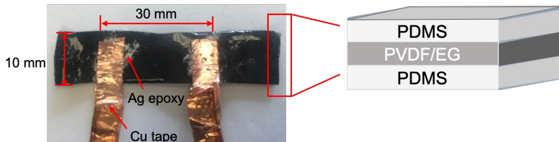
Fig. 31: Dimension and structure of the thin film sensor
