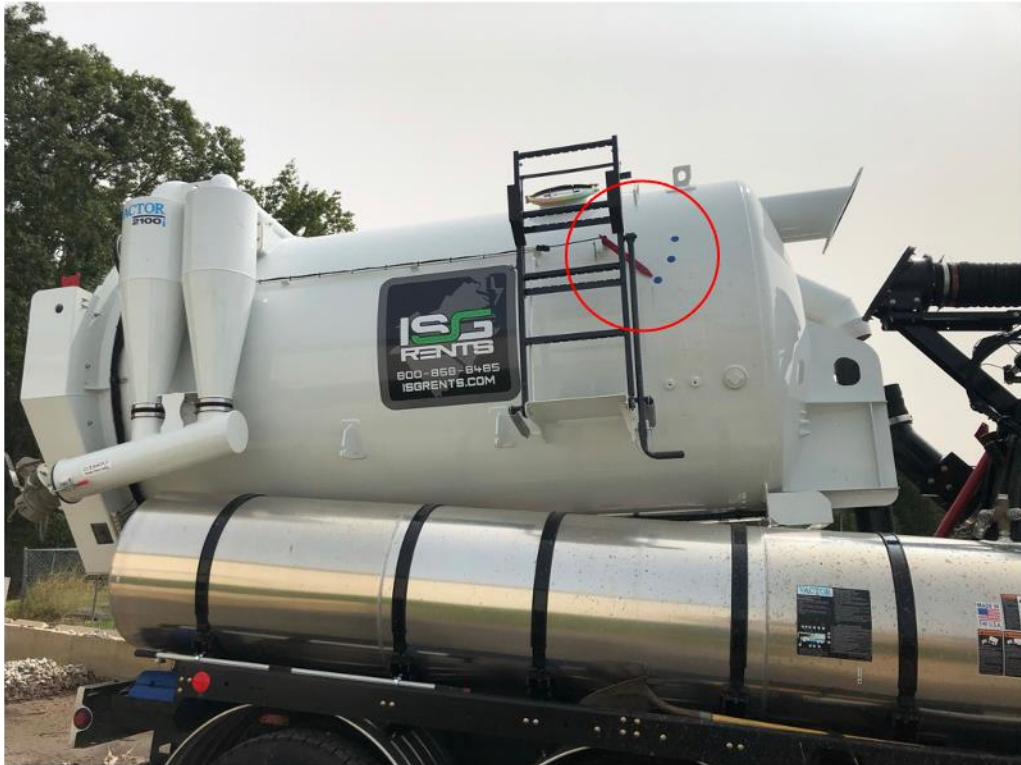
Figure 8. Side View of a Typical Vacuum Truck With Available Capacity Indicator Circled in Red
