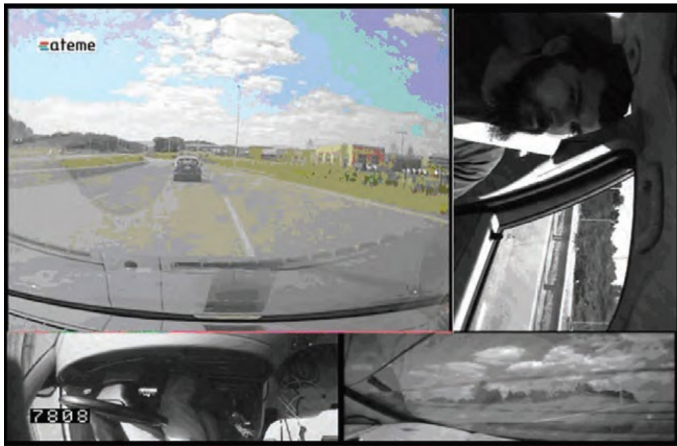
Figure 7. Screen capture. SHRP 2 camera views: forward view (upper left), the driver's face (upper right), downward view of drivers' hands on the steering wheel (lower left), and rear view (lower right).
