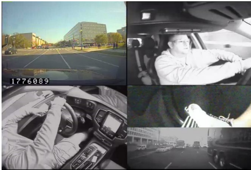
Figure 8. Screen capture. SMX camera views: forward view (upper left), the driver's face (upper right), downward view of the instrument panel and the drivers' hands on the steering wheel (lower left), foot on the brake (middle right), and rear view (lower right).
