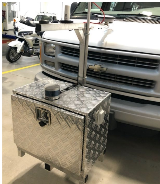
Figure 5. Photo. LV package installed on the front hitch of a VTTI fleet vehicle.
