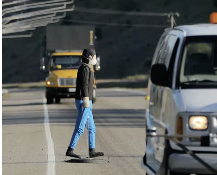
Figure 7. Photo. Object detection testing with the VTTI robot.
