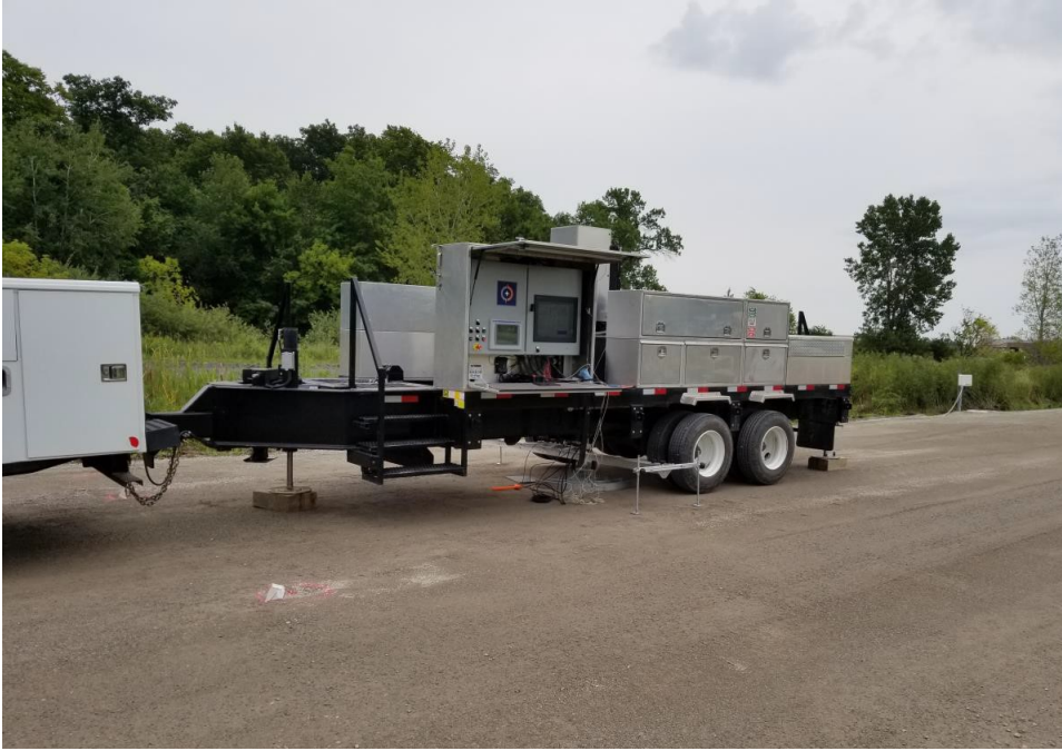
APLT test system at the MnROAD LVR (White and Vennapusa 2017):
