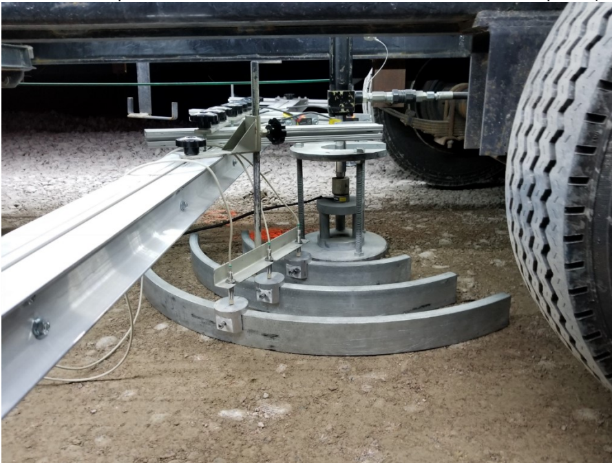
APLT test setup and deflection basin measurement kit with center plate (White and Vennapusa 2017):
