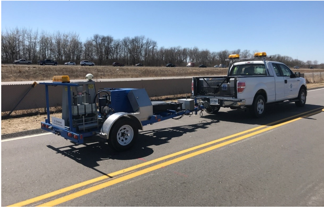
Trailer-mounted Dynatest Model 8002 FWD device:
