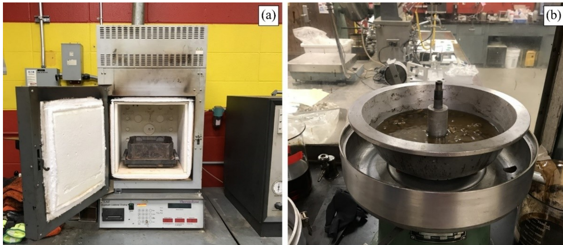
Figure 4.4. (a) Ignition furnace used in ignition method and (b) asphalt extraction bowl used in quantitative extraction
