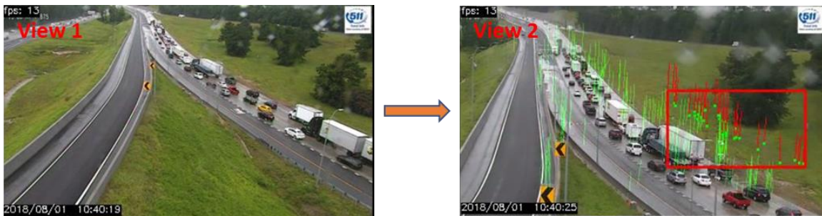
(a) Incident alarms for wrong-way driving are likely to be generated when there is a shift in camera view in a Pan-Tilt-Zoom camera.
