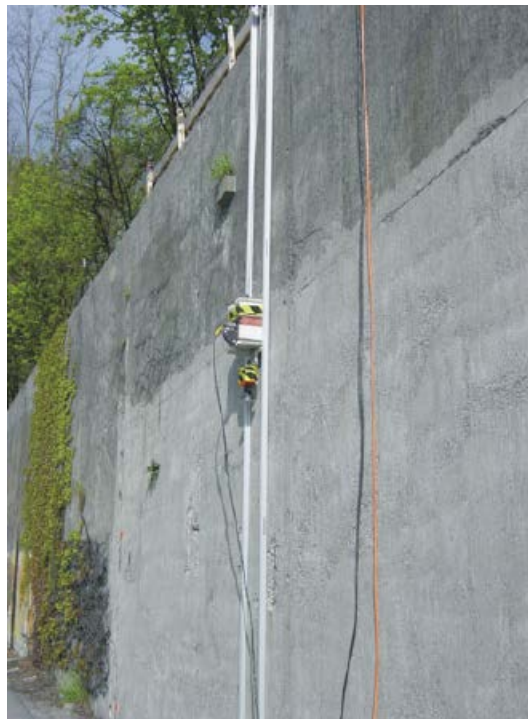
Figure 1.12. Semi-automated survey apparatus (from Hugenschmidt and Kalogeropoulos 2009)
