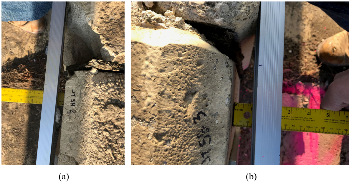
Figure B.1. Manually measured movement of the M-10 wall panel at the top wall parapet in January 2020.
