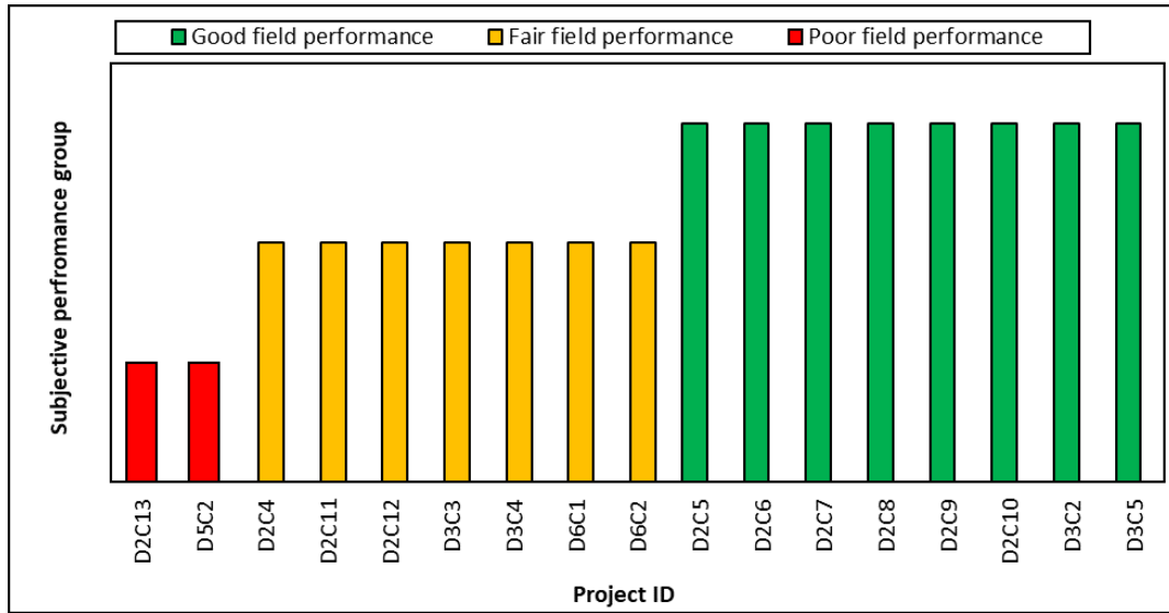
Figure 29 Cracking Resistance Evaluation for all Field Test Projects
