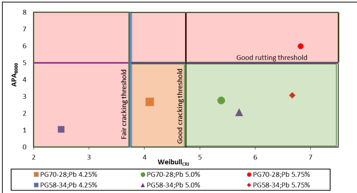
Figure 137 Implementation of Performance Tests as Part of Superpave Design Method
