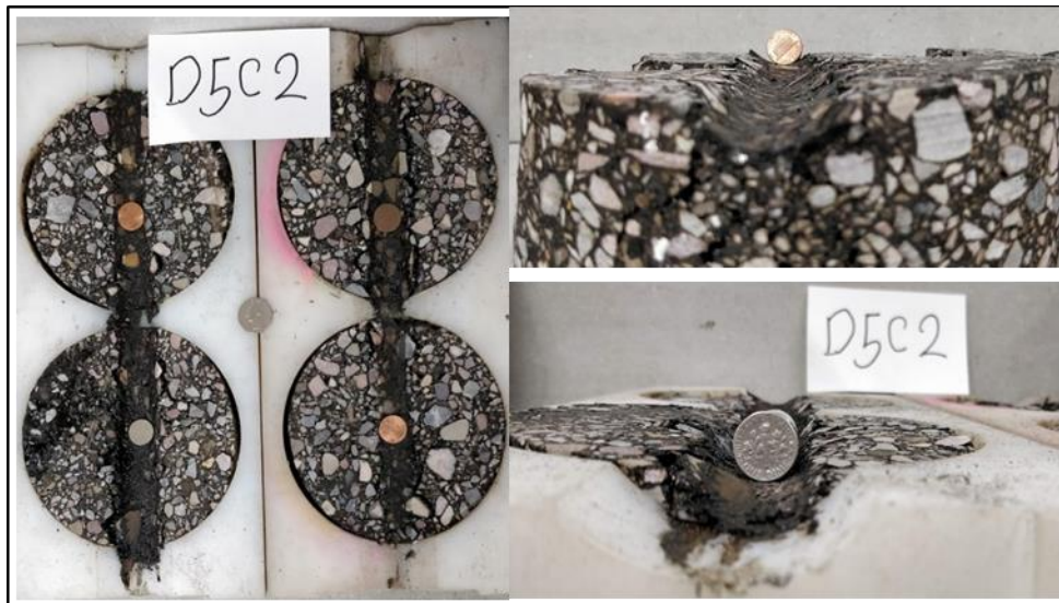
Figure 121 Mixture D5C2 Specimens after Testing using APA Test
