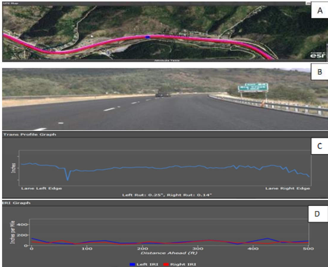
Figure 26 PathRunner Outputs for D1C1 between MP 53 and MP 54; (a) GPS Route Map (b) Road Perspective, (c) Rut Depth Profile (d) IRI Profile
