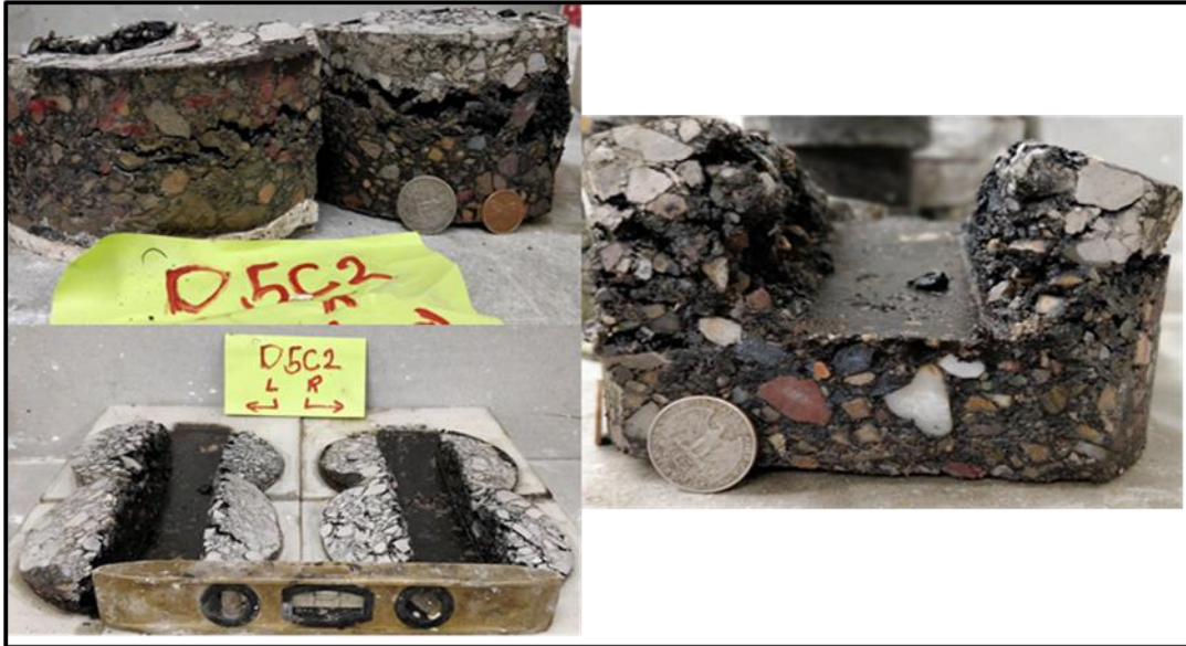
Figure 118 Mixture D5C2 Specimens after Testing using HWTT Test
