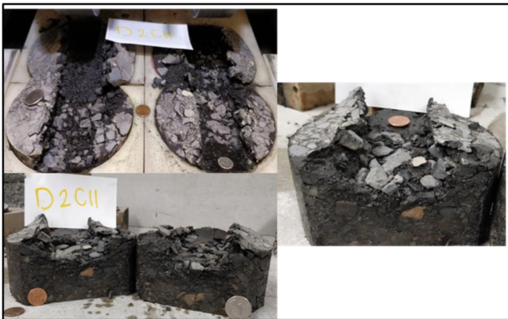
Figure 119 Mixture D2C11 Specimens after Testing using HWTT Test
