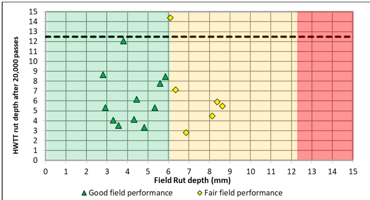
Figure 123 Laboratory HWTT Rut Depth after 20,000 Passes versus Field Performance
