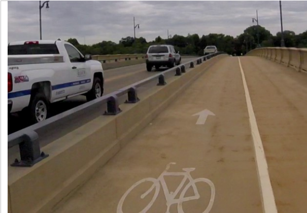
Buffer 1: Wall or Tall Barrier (impenetrable)
