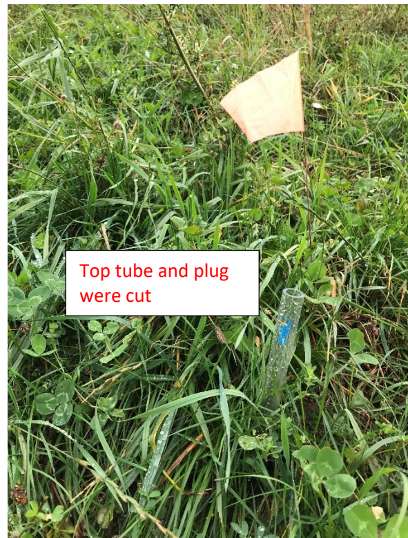
Figure 2.9 Pictures of destroyed lysimeters taken on October 11, 2019. The picture of a working lysimeter is shown on the left in Figure 2.7.
