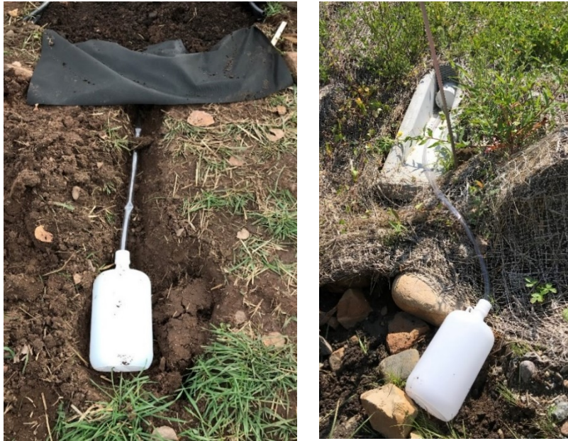
Figure 2.6 Perforated pipe to collect water samples in the NRRI site (left) and Eagle's Nest trench site (right).
