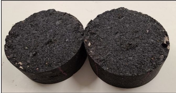
Figure 6.6: A specimen that failed along the tack coat interface.
