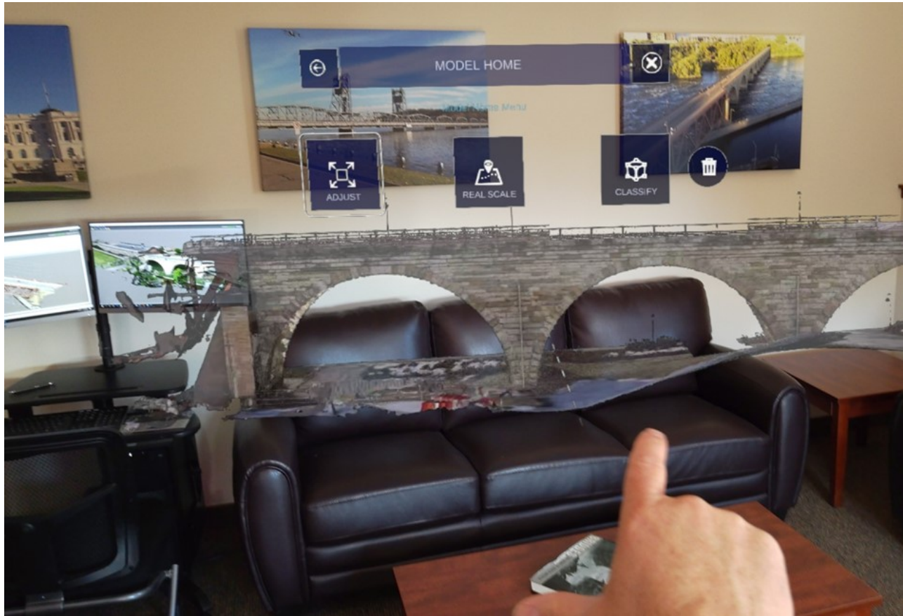
Figure 4-39 Virtual Inspection of Bridge Using Microsoft Hololens 2
