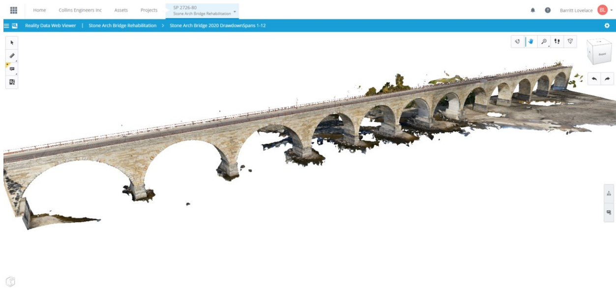
Figure 4-33 3D Reality Model of Stone Arch Bridge During River Drawdown
