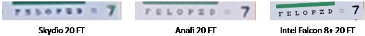
Figure 2-34 Comparison of the Three Cameras at 20 Feet for Line 7 of the Optical Vision Test
