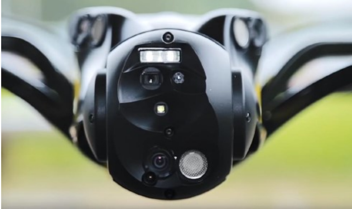
Figure 2-13 Sensefly Albris TripleView Payload
