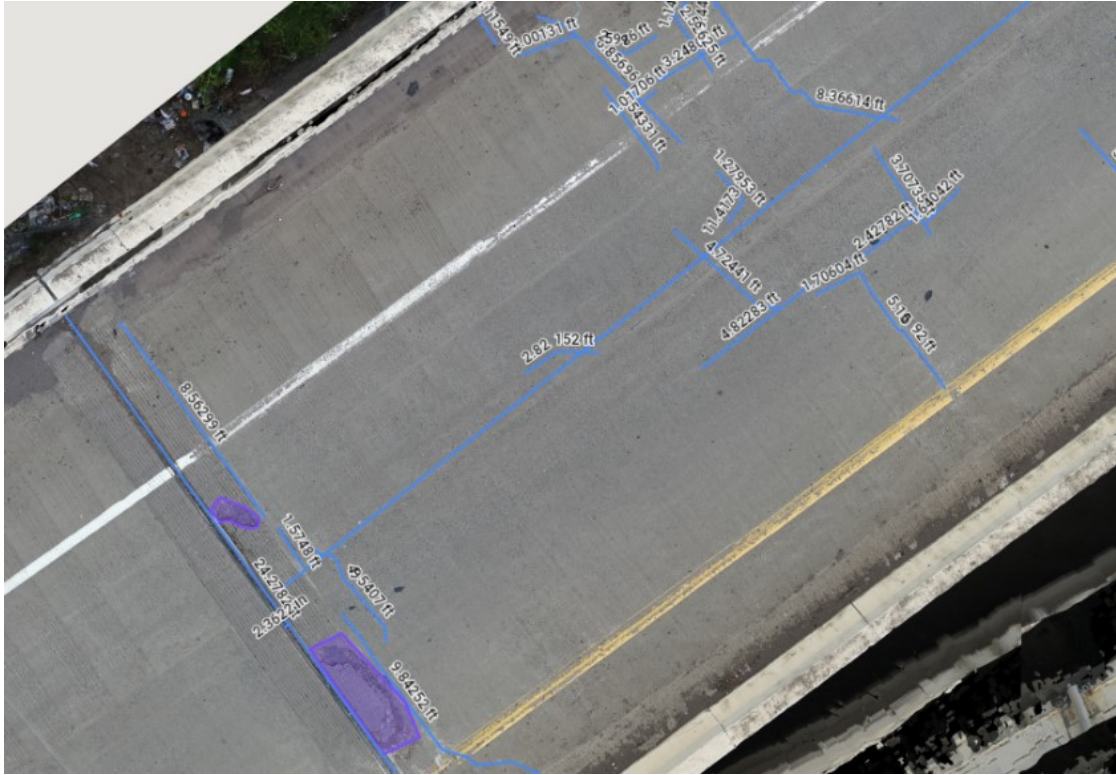
Figure 4-7 Bridge 27831A Deck with Measurements in Pix4D Cloud
