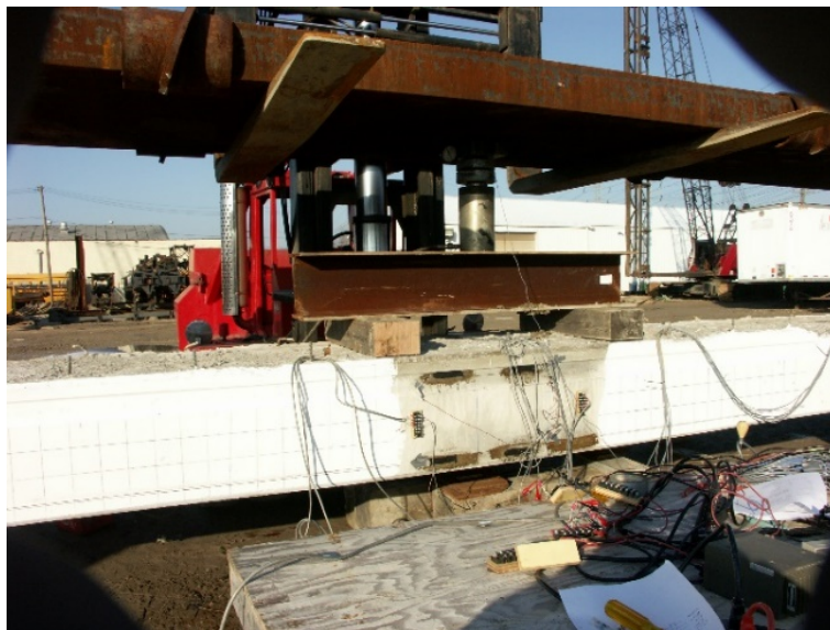
Figure 2-14. Load test setup for four-point bending test
