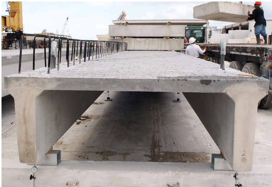
Figure 2-10. Load testing of a double tee beam at the fabricator's yard (Spadea et al. 2018)
