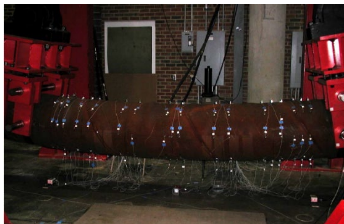
Figure 2-21. Reversed cyclic testing of a pile (NDI 2020)
