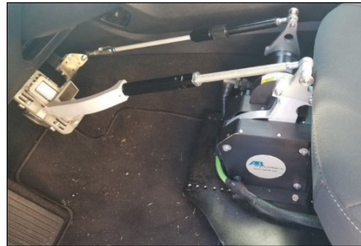
Figure 2-9: Example of a robotic brake and throttle controller installation.
