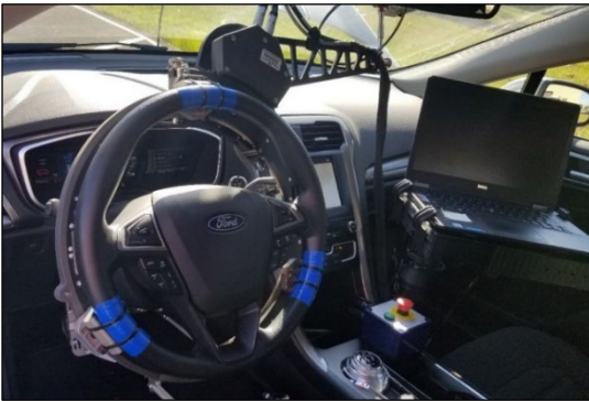
Figure 2-8: Example of a robotic steering controller installation.
