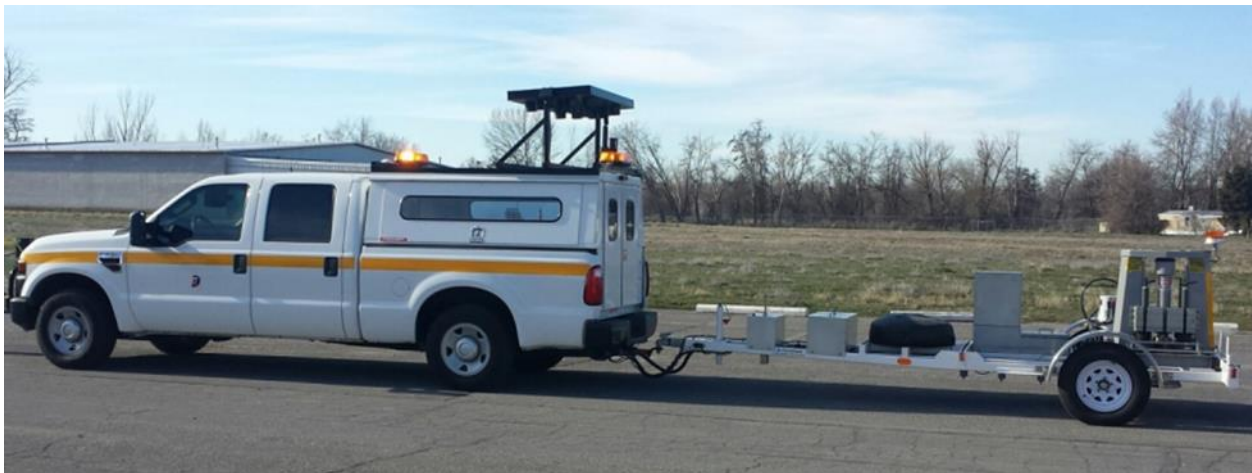
Figure 1: ITD's FWD Truck and Trailer
