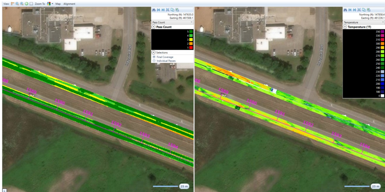
Figure 3.1 Example map of intelligent compaction (left) and paver mounted thermal profiling data (right) in Veta.
