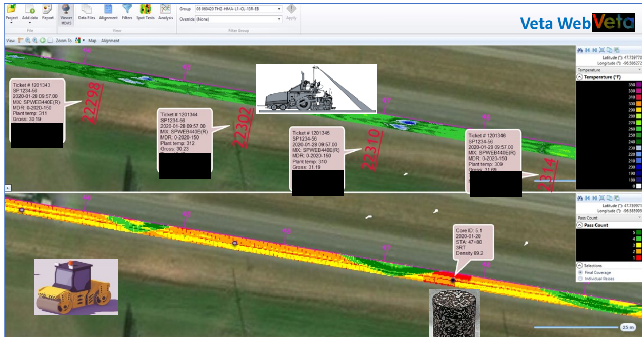
Figure 3.3 Example Mark-Up of E-Ticket with Respect to IC and PMTP Data in Veta Web.
