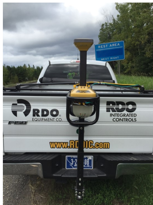
Figure 1.2 Image of RD-M1 system mounted to a truck.
