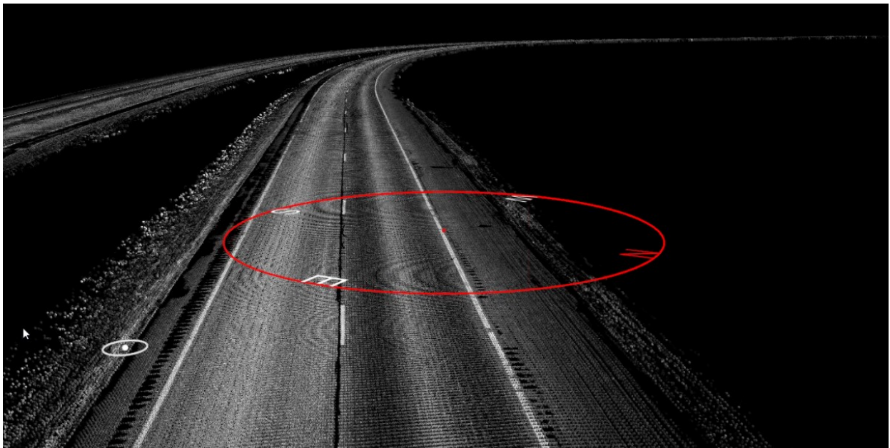
Figure 1.8 Example of features collected when viewing in black and white within Topcon Magnet Collage.
