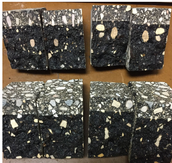
Figure 18. Fracture of aggregate at cracking interface using the modified TP105 SCB procedure.
