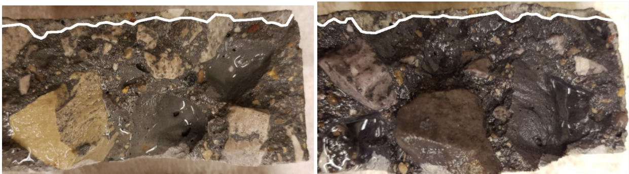
Figure 4.4 Example Depth of Penetration for SME-PS Specimen (Left: water, Right: blue fabric dye)
