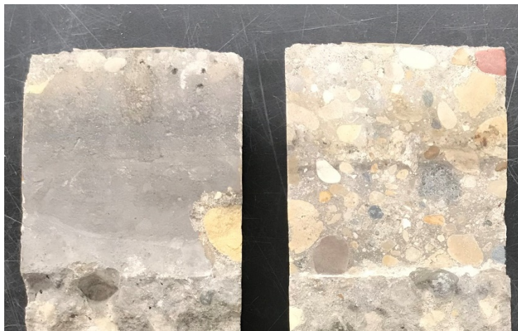
Figure 5.7 Silane-treated core sample (left) as received and (right) after cleaning
