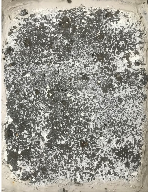
Figure C.8 FA Lithium Silicate mixture applied moist after 30 minutes after 50 Cycles
