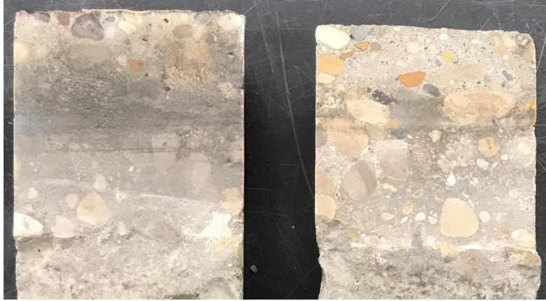
Figure 5.6 Untreated core samples (left) as received and (right) after cleaning
