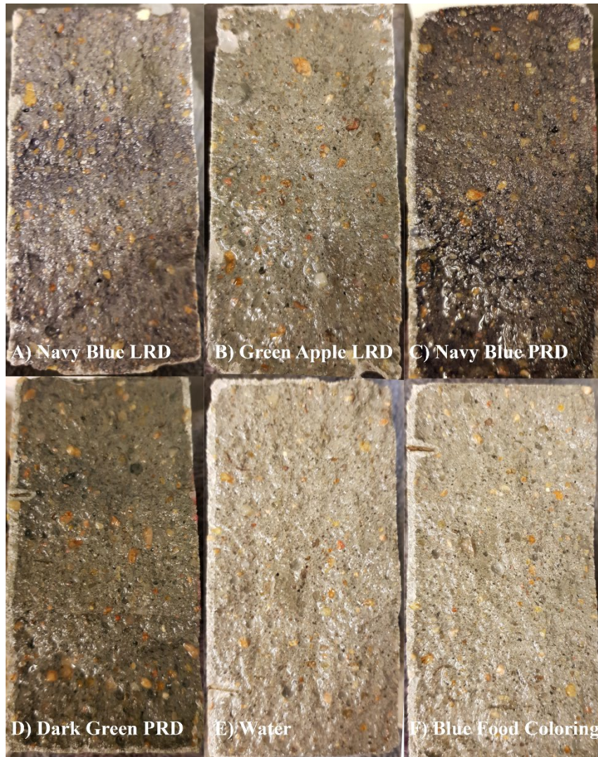
Figure C.3 Secondary Dye Testing for Depth of Penetration
