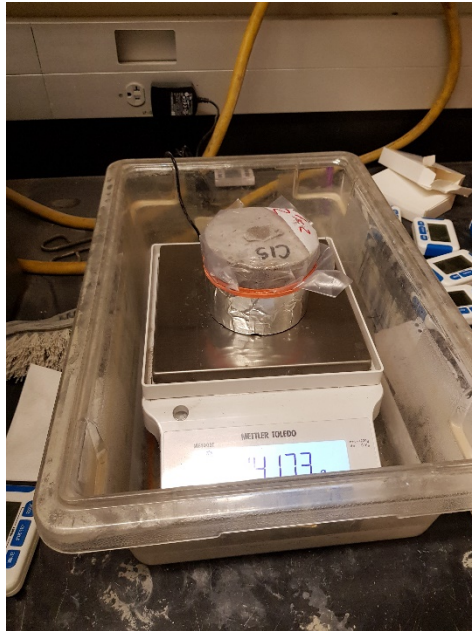
Figure 3.4 Lab setup for absorption test of core samples
