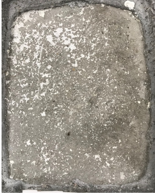
Figure C.6 FA Silane applied moist after 30 minutes after 50 Cycles
