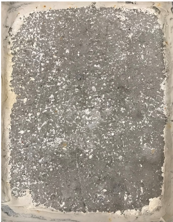
Figure C.5 FA Silane applied dry after 50 Cycles
