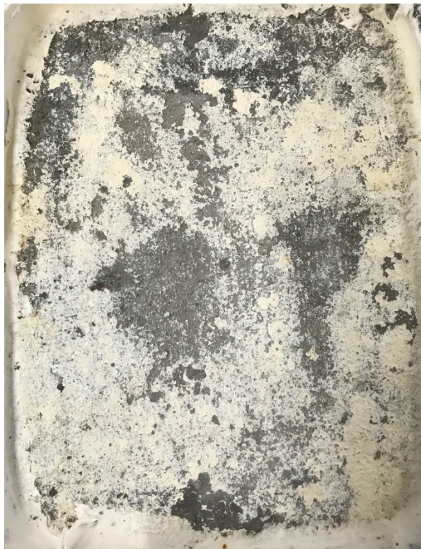
Figure C.7 FA SME-PS applied dry after 50 Cycles
