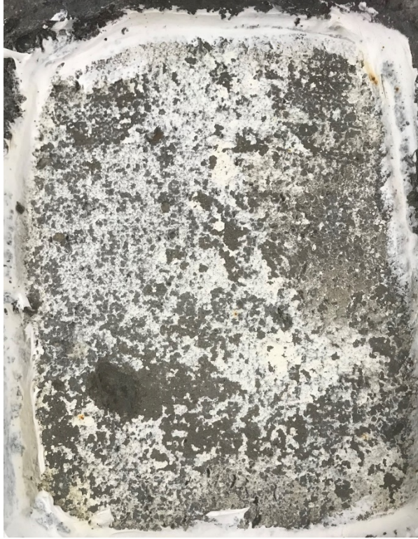
Figure C.4 FA Control after 50 Cycles
